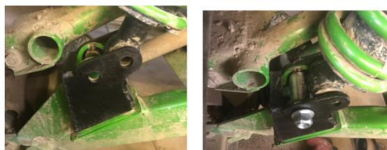
Once your Spacer and bracket are in place, along with the mounting bolt, its time to install the Lower shock mounting bolt and the “Fat Washers”.. Install 1 fat washer on each side of the lower shock mount, this will take up the void area that the lift bracket has created. You can also install the lower shock mounting bolt from the “Axle side” as well. This will put both nuts towards the rear of the machine and make it easier for tightening later in the process.
