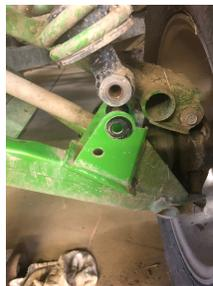
A suggestion that will also help aid the installation of your bracket, as well as allow the shock to positions it self easier, is to loosen the upper shock mounting bolt as well. To do this, you'll need a 17MM socket and Wrench combination. It can also be done using and impact gun as well.
