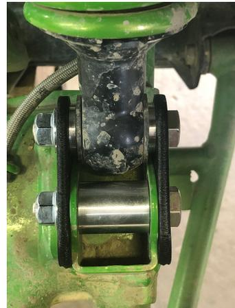
If you'll be adjusting the preload, please refer to the steps outlined in the rear bracket installation process. **That front is adjusted in the same manner, but instead, the preload is adjusted to 9-7/8"**. Some users have stated that 9-3/4 is also a good baseline setting.
