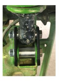
If you'll be adjusting the preload, please refer to the steps outlined in the rear bracket installation process. **That front is adjusted in the same manner, but instead, the preload is adjusted to 9-7/8".** Some users have stated that 9-3/4 is also a good baseline setting.
