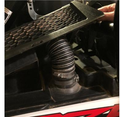
**STEP 5.** Install Particle Separator (1) onto the Metal Brackets (5) on the left and right side using Screw (6) and Washer (4) and a 3/16" Hex Key to tighten. Washer **MUST** be between the Metal Bracket (5) and Particle Separator (1). If the washer is placed under the head of the Screw (6) the Particle Separator will rotate freely and may cause damage.
