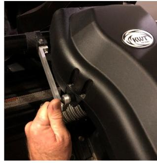
**STEP 6.** If necessary cut excess off the Flexible Duct (9) with wire cutters for better fit. Insert the Hose Clamp (2) over the end of the Flexible Duct (9) that is sticking out of the Air Intake cover. Place the Flexible Duct (9) over the Particle Separator (1) intake and tighten with a Philips screwdriver.
