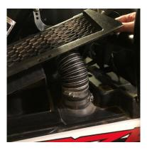
**STEP 5.** Install Particle Separator (1) onto the Metal Brackets (5) on the left and right side using Screw (6) and Washer (4) and a 3/16" Hex Key to tighten. Washer **MUST** be between the Metal Bracket (5) and Particle Separator (1). If the washer is placed under the head of the Screw (6) the Particle Separator will rotate freely and may cause damage.
