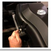
**STEP 6.** If necessary cut excess off the Flexible Duct (9) with wire cutters for better fit. Insert the Hose Clamp (2) over the end of the Flexible Duct (9) that is sticking out of the Air Intake cover. Place the Flexible Duct (9) over the Particle Separator (1) intake and tighten with a Philips screwdriver.
