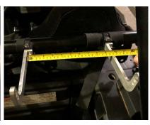
**STEP 3.** Take the stock Air Intake Cover and measure a hole that will align with the air intake. Cut a 3" hole using a 3.25 diameter hole saw or trim using a dremel. Install included rubber stripping around the hole in the Air Intake Cover. Insert the Flexible Hose Duct (9) through the Air Intake Cover and insert two Hose Clamps (2) over the end of the Flexible Hose Duct (9)
