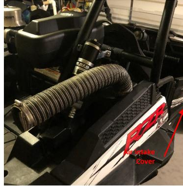
**STEP 7.** Install Particle Separator (1) onto the Metal Brackets (5) on the left and right side using Screw (6) and Washer (4) and a 3/16" Hex Key to tighten. Washer **MUST** be between the Metal Bracket (5) and Particle Separator (1). If the washer is placed under the head of the Screw (6) the Particle Separator will rotate freely and may cause damage.
