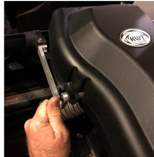
**STEP 8.** If necessary cut excess off the Flexible Duct (9) with wire cutters for better fit. Insert the Hose Clamp (2) over the end of the Flexible Duct (9) that is sticking out of the Air Intake cover. Place the Flexible Duct (9) over the Particle Separator (1) intake and tighten with a Philips screwdriver.
