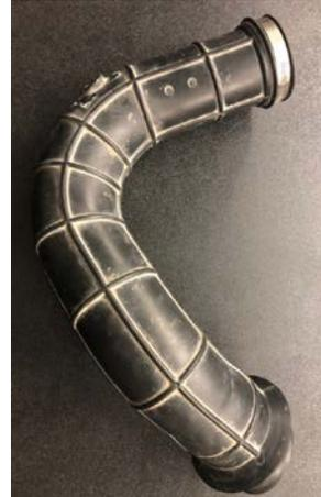
**STEP 5.** Locate the Flexible Hose Duct (ITEM 8, page 4) within the KWT installation kit. Insert the flexible hose duct (Item 8, Page 4) onto the stock RZR Filter Air Box intake side and tighten the Hose Clamp (ITEM 2) (shown below).
