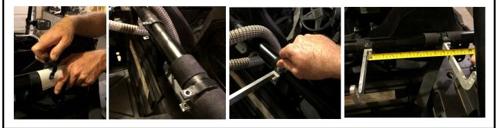
**STEP 3.** Take the stock Air Intake Cover and measure a hole that will align with the air intake. Cut a 3.5" hole using a 3.50 diameter hole saw or trim using a dremel. Install included rubber stripping around the hole in the Air Intake Cover. Insert the Flexible Hose Duct (9) through the Air Intake Cover and insert two Hose Clamps (2) over the end of the Flexible Hose Duct (9)
