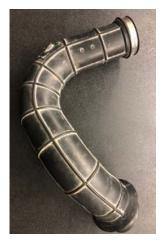
**STEP 5.** Locate the Flexible Hose Duct (ITEM 8, page 4) within the KWT installation kit. Insert the flexible hose duct (Item 8, Page 4) onto the stock RZR Filter Air Box intake side and tighten the Hose Clamp (ITEM 2) (shown below).
