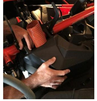
**STEP 5.** Install Particle Separator (1) onto the Metal Brackets (5) on the left and right side using Screw (6) and Washer (4) and a 3/16" allen wrench to tighten. Washer **MUST** be between the Metal Bracket (5) and Particle Separator (1). If the washer is placed under the head of the Screw (6) the Particle Separator will rotate freely and may cause damage.
