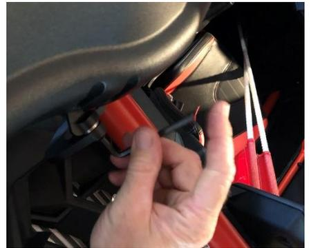
**STEP 6.** If necessary, cut excess off the Flexible Duct (9) with wire cutters for better fit. Insert the Hose Clamp (2) over the end of the Flexible Duct (9) that is sticking out of the Air Intake cover. Place the Flexible Duct (9) over the Particle Separator (1) intake and tighten with a Philips screwdriver.
