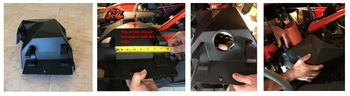
**STEP 5.** Install Particle Separator (1) onto the Metal Brackets (5) on the left and right side using Screw (6) and Washer (4) and a 3/16" allan wrench to tighten. Washer **MUST** be between the Metal Bracket (5) and Particle Separator (1). If the washer is placed under the head of the Screw (6) the Particle Separator will rotate freely and may cause damage.
