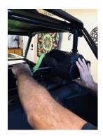
**STEP 6.** Measure Flexible Duct (9) to Particle Separator (1) inlet, if necessary, cut excess off the Flexible Duct (9) with wire cutters for better fit. Insert the Hose Clamp (2) over the end of the Flexible Duct (9) that is sticking out of the air intake panel. Place the Flexible Duct (9) over the Particle Separator (1) intake and tighten Hose Clamp (2) with a Philips screwdriver. Once completed replace all side plastics back onto the vehicle.
