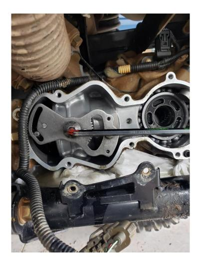
Install the new gear and new pin into the diff.
