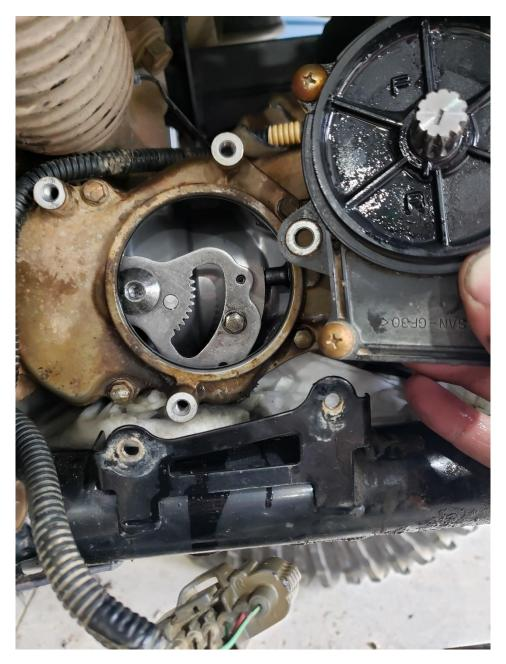
Install the axle and before putting everything back together check actuation of 2-wheel drive, 4-wheel drive and diff lock. Rotating the axle may be necessary to get the gear to line up with the receiving carrier
