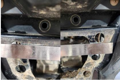
THE TOP OF THE WINCH MOUNT WILL FEED THRU AND HOOK ON THE BACKSIDE OF THE FRAME RAIL
