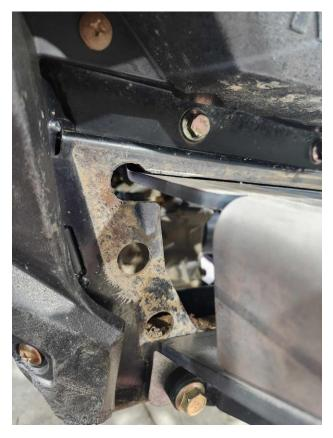
THE BOTTOM OF THE MOUNT WILL BOLT TO WHERE A PULL POINT WOULD GO. HARDWARE IS LONG ENOUGH TO USE WITH OR WITHOUT A PULL POINT
