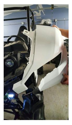
Once you've removed the fenders you'll need to remove the front grill. There are a few screws and push pins holding it on.
