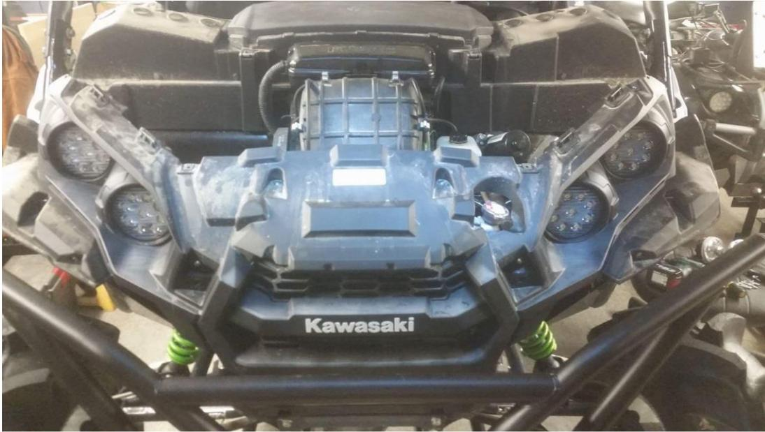
When proper positioning is achieved, tighten all the mounting bolts to the headlights.
