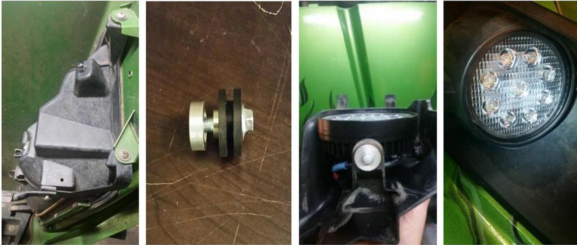
Remove two bolts to reveal headlight housing. FIG: 1
