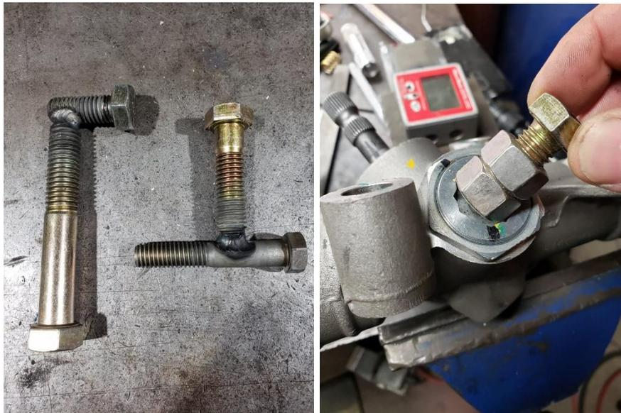
It is easier to loosen the jam nut first and unscrew the assembly.
