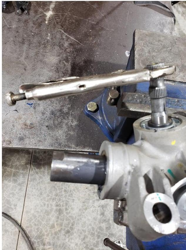
Once the rack is out of the machine you can disassemble the jam nut and cap
