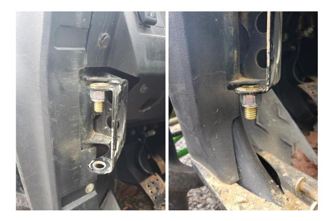
The smaller bolts will bolt onto the door frame itself
