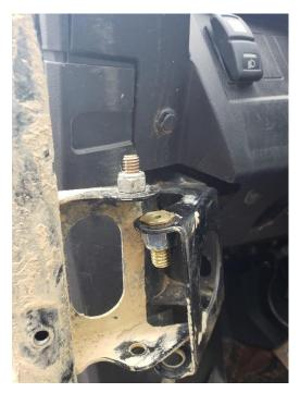
Insert the new pins and be careful not to lose the small c clips that hold the pin in place.
