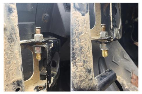
with this bushing design you are not using all four "pivot" locations just the very top and the very bottom Two bushings sets and two pins are used for one door
