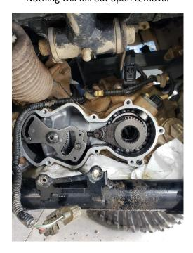
Remove the shift fork pin to remove the gear and shift fork
