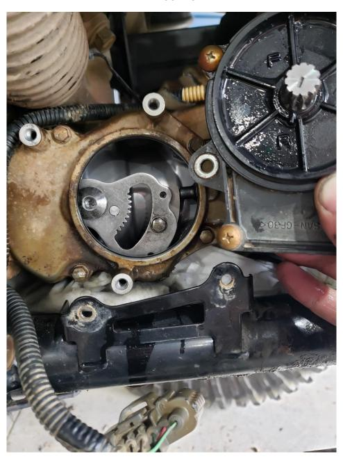
Install the axle and before putting everything back together check actuation of 2-wheel drive, 4-wheel drive and diff lock.
