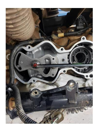
Install the new gear and new pin into the diff.
