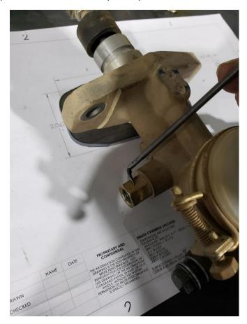
You will reuse the banjo bolt, hardline adapter, firewall bolts and the clevis pin on the brake petal
