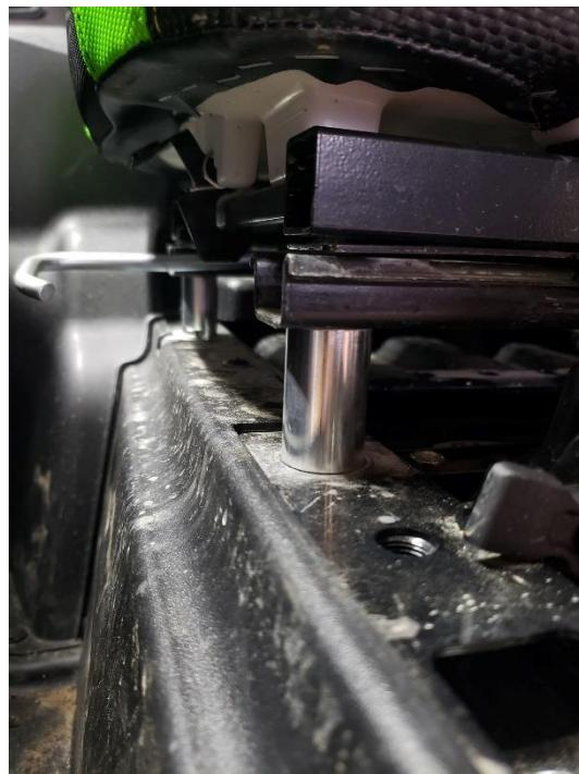
Spacers will install under the seat frame rail with longer hardware provided
