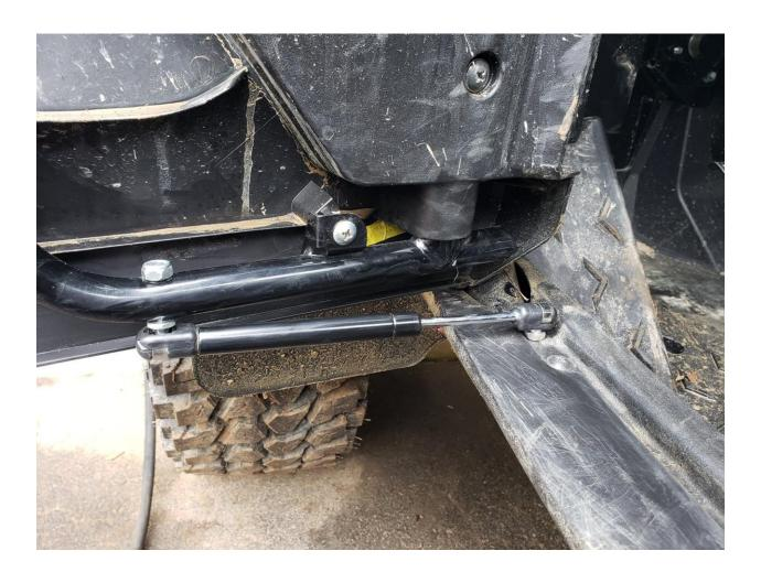
$\frac{\text{First}}{\text{measure 1" from the center of the floorboard screw}}$  Drill and tap a hole to accept the short ball stud. Install stud
