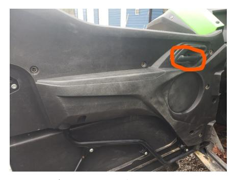
Start by removing all the screws/push pins in the door frame and the two bolts that hold the latch to the door
