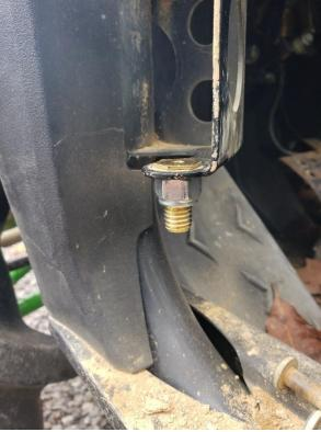
The smaller bolts will bolt onto the door frame itself
