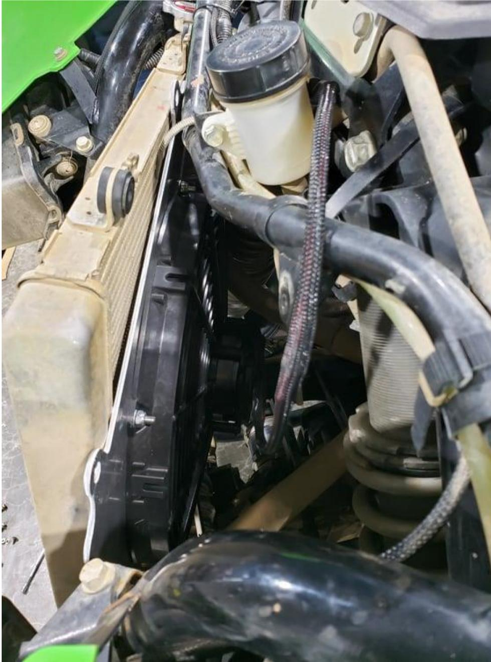
Align the new fan assembly so no edges are rubbing the radiator
