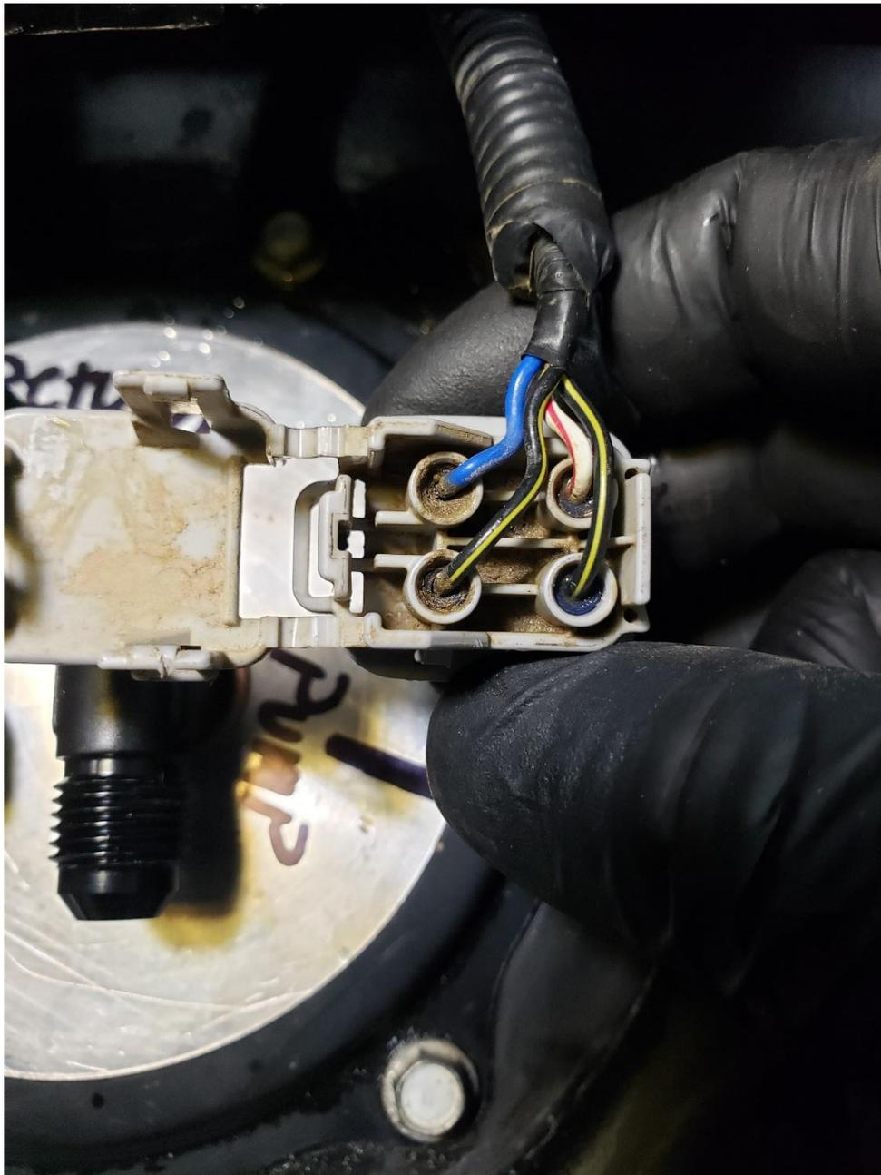
Install the terminals in the new connector as shown
