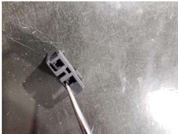
Insert the terminals into the new connector provided
