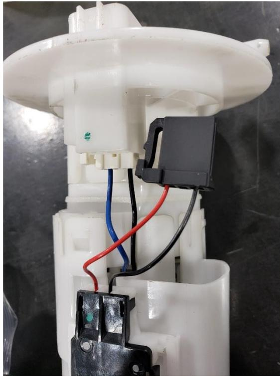
Unpin the connector from the wiring
