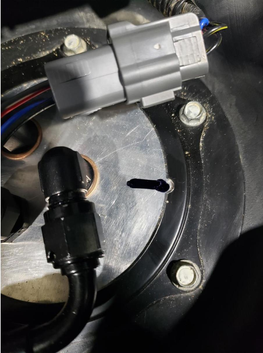
Next you will re pin the machine side of the fuel pump connector
