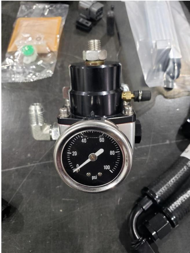
Install the line from the fuel rail to the 90 fitting on the regulator
