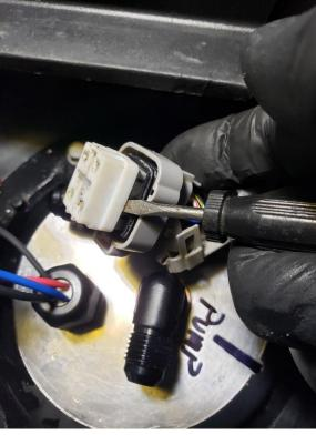
Using the pick remove the terminals from the connector housing
