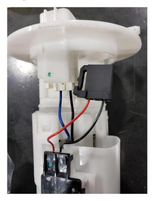
Unpin the connector from the wiring
