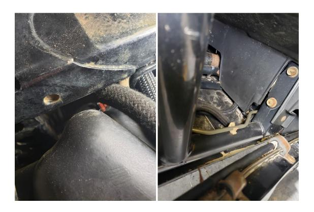
Run your hose from the fuel filter and follow the stock fuel line up to the fuel rail
