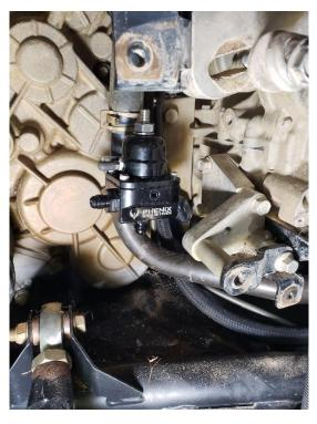
Drill a ¼ inch hole in the bracket as shown and install the regulator with nut and bolt provided
