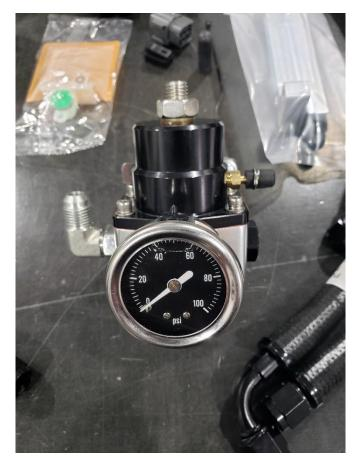
Install the line from the fuel rail to the 90 fitting on the regulator
