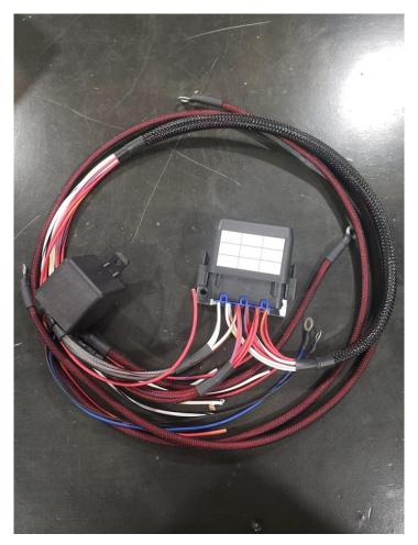
Fuse block is setup for 5 constant fused sources and 4 switched sources.
