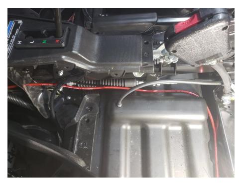
The long main power wire gets attached to the battery
