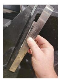
The spring hinge will need to be positioned flush with the outside plastics
