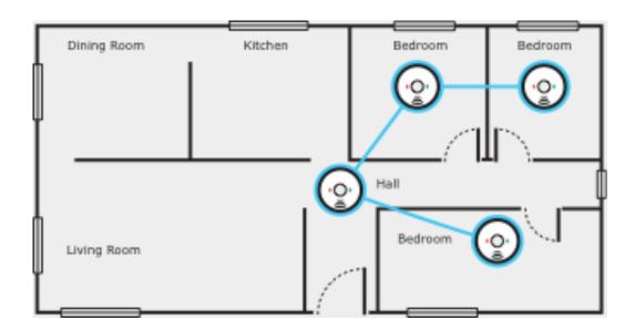
Where practicable smoke alarms must be placed on the ceiling.
