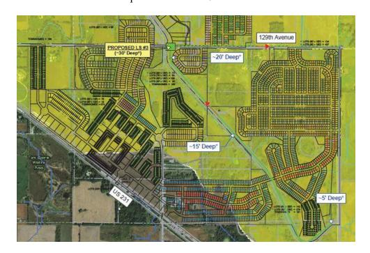
In Exhibit 8, on the other hand, Winfield depicts flows traveling southeast along U.S. 231 via gravity sewer to proposed Lift Station # 2 (south of the Development Area). From there, flows travel north by force main to proposed Lift Station # 1 as shown in the excerpt from Exhibit 8 below.
