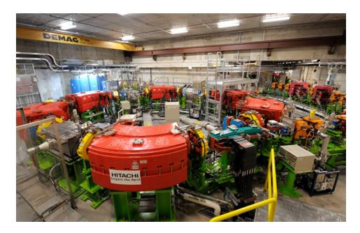
The photo below illustrates how the accelerator is deployed to each of the four-treatment room. The red images in these pictures are magnets used to energize the particles. The pipes then carry the proton energy to each of the four treatment rooms here at the Clinic through a series of pipes as seen in this picture. The treatment room can be seen in the long corridor extending to the right of the photo.
