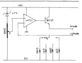
FIG. 1. Electrical circuit of the current source. The direct current is produced by a current source, which is supplied by two 9-V batteries. An operational amplifier ( $\mu P$  741) assures each required current to be kept constant. The value of the output current is controlled by potentiometer (P) and range switch (S).
