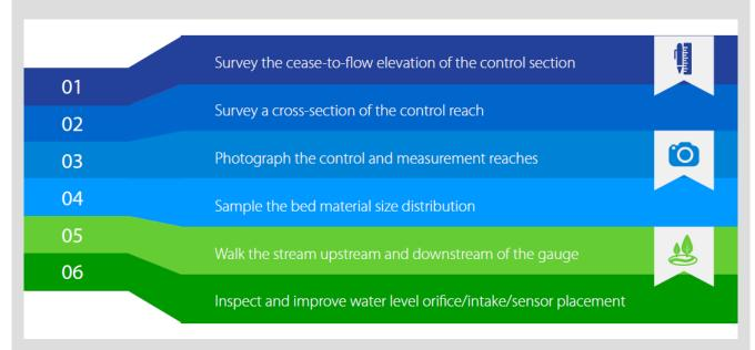
As Civil Engineers are recording some of the lowest flows in the past century, it is an excellent time to conduct replicate gaugings. Changing equipment and/or initial point for soundings provides a wealth of information that is helpful for accurate calibration of the low end of the rating curve. In the time it would take to do one high flow gauging it may be possible to do several low flow gaugings.
