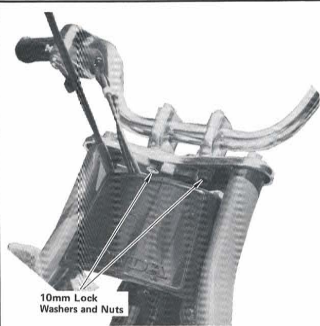
STEP 11 —Install handlebar on upper fork bridge as shown using two 10mm lock washers and nuts. Tighten nuts to specified torque.
