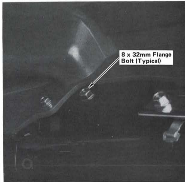
STEP 39 —Position rear carrier on frame as shown and install using an 8 x 32mm flange bolt on each side.
