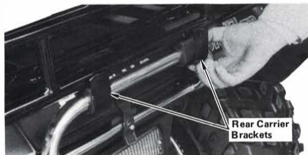
STEP 40 —Install carrying handle rubbers on carrying handle as shown and slip a rear carrier bracket over each rubber as shown.
