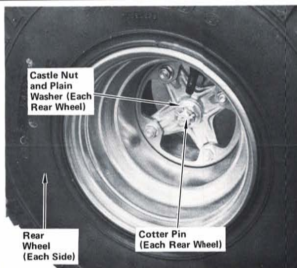
STEP 37 —Grease rear axle splines and install rear wheels, with valve stems to the outside, using a plain washer and castle nut for each. Tighten both castle nuts equally to specified torque and install a cotter pin in each. Spread ends of cotter pins as shown.
