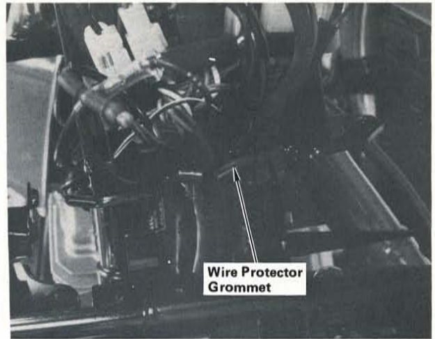
STEP 55 —Insert the connector wires into the two holes of the wire protector grommet, and install the grommet on the bottom of the connector bracket as shown.
