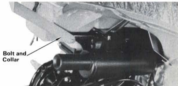
STEP 8 —Remove the front shipping bracket by loosening fork bolts. Retighten bolts to the specified torque. Remove the rear shipping bracket by removing the bolt and collar. Discard bolts, brackets and collar.
