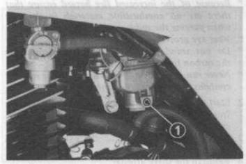
(1) Carburetor drain bolt
