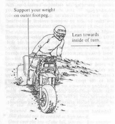
Incorrect turning techniques may cause the front wheel to slide straight ahead when steered without affecting the ATC's direction of travel. If this should occur, close the throttle and come to a stop. Then continue practicing the technique outlined on the preceding page.
