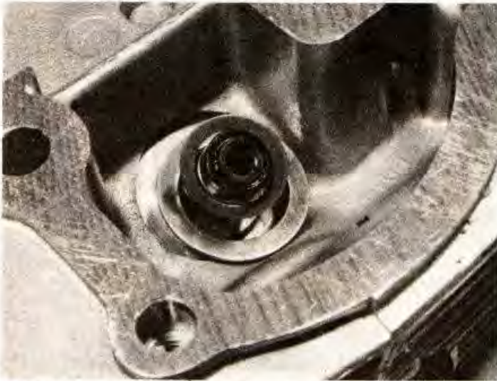
4.123 Be sure to install both the inner and outer spring seats before assembling the valves and springs
