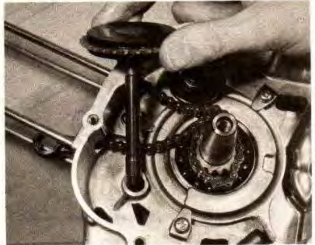
14.2 Draw out the oil pump drive shaft and sprocket (ATC 90/110)
