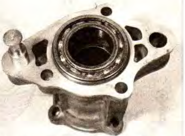
7.5b Bearings should be tapped out and renewed if worn
