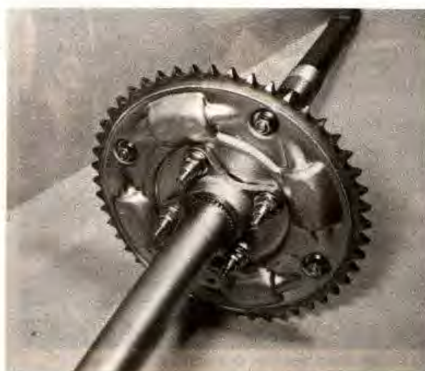
10.11b Re-install sprocket assembly after checking condition of retaining bolts and nuts
