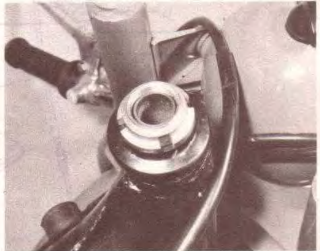
6.3a Adjust steering head bearings using a C-spanner on this adjuster nut
