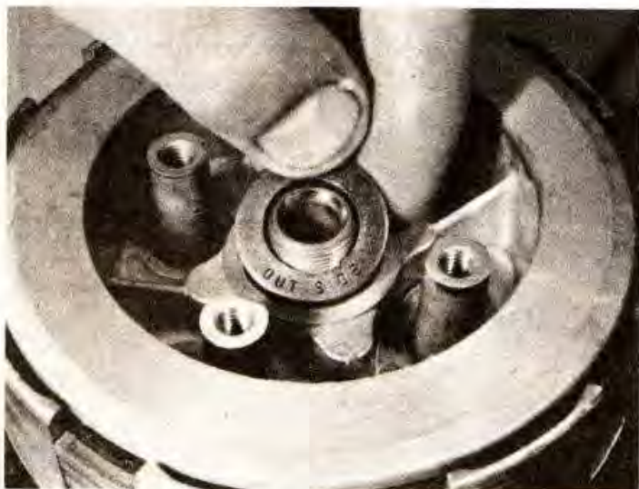
4.217 The lockwasher must be installed with the marked side out
