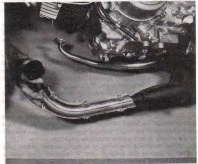
52.5a Refit the exhaust system using a new flange gasket and
