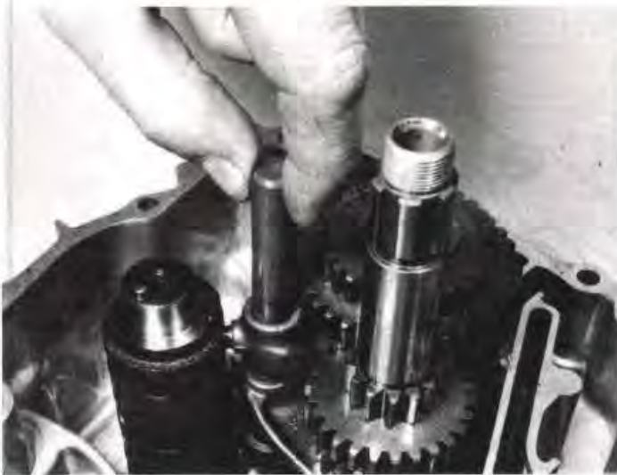
4.194 Installing the selector fork shaft
