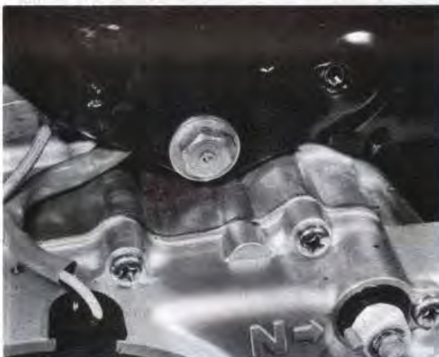
5.12a Remove the upper rear bolt ...
