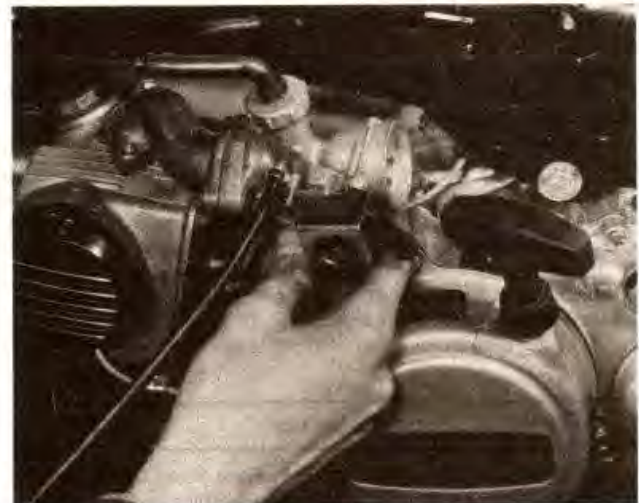
6.6 Removal of the two flange nuts now allows removal of carburettor
