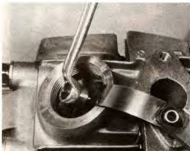
Set clearance so that the feeler gauge is a sliding fit
