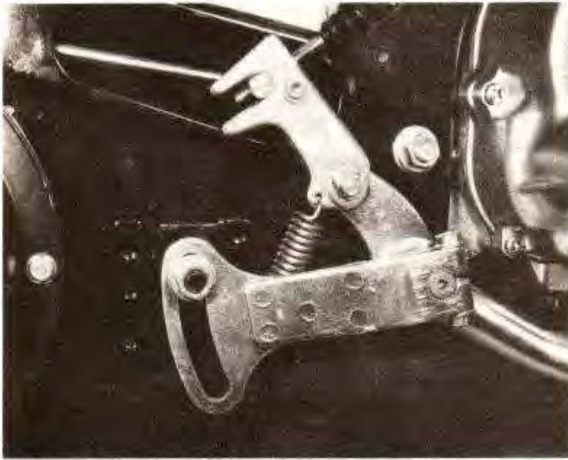
11.4a Loosen chain tensioner locking nut and push arm upwards until resistance is felt, indicating that ...
