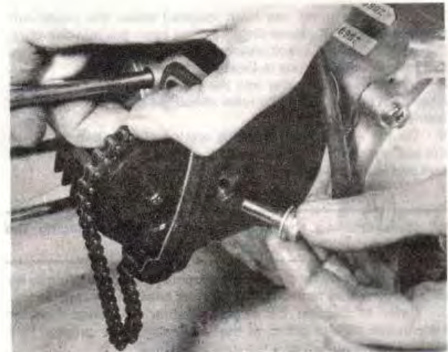
47.8 Refit and secure the cam chain guide roller
