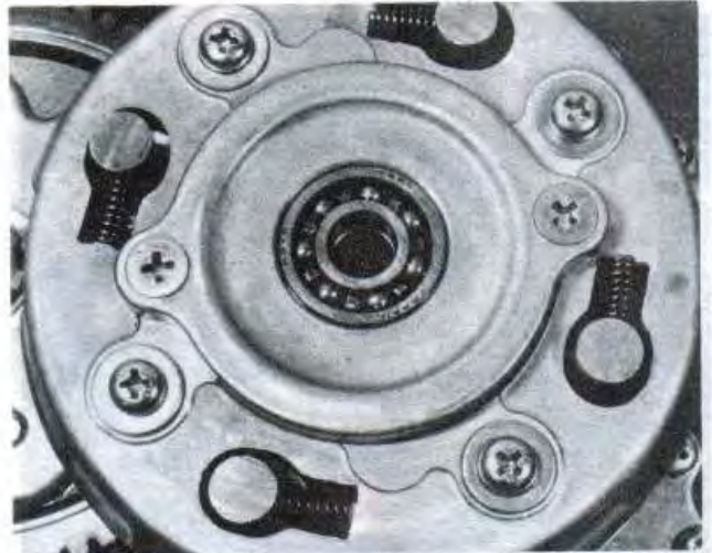
10.4 Remove the clutch outer cover and centre bearing/centrifugal oil filter
