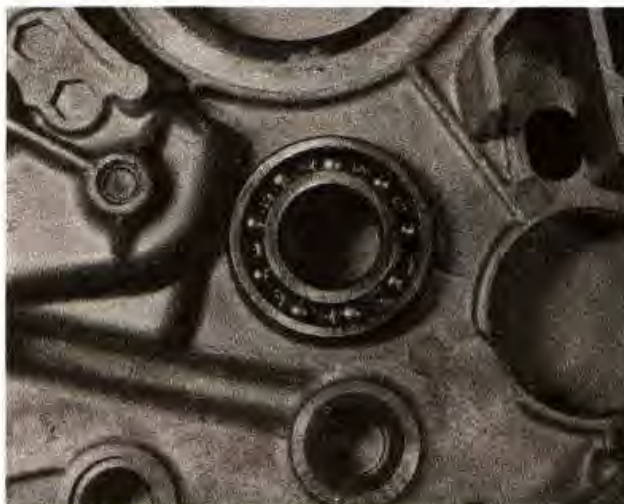
37.1 Bearings can be driven home using a suitable drift
