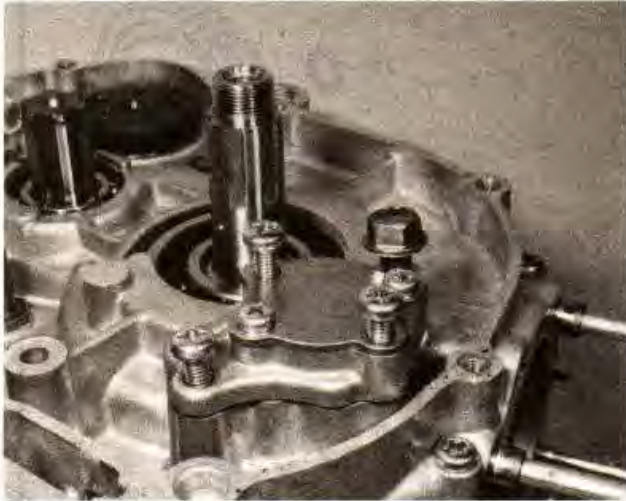
11.1 Remove three screws and special bolt (ATC 90/110) to release oil pump
