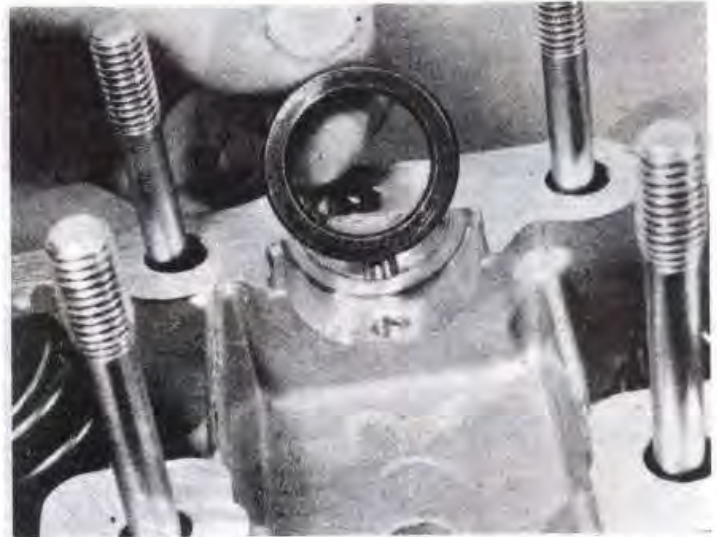
4.253 Installing the camshaft bushing (make sure the locating pin on the bushing fits into the hole in the bearing recess)
