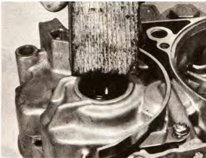
4.85b When installing new oil seals, carefully drive them into position with a block of wood or a large socket
