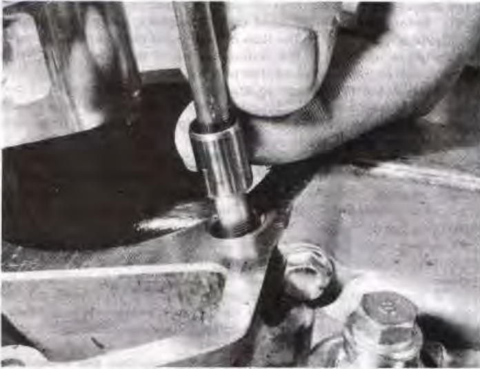
4.241 Be sure to install the dowel pins on the left side cylinder studs
