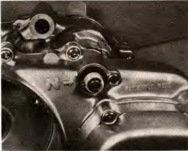
45.5 Exterior end of neutral indicator device is retained by small 'E' clip
