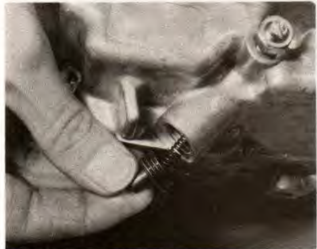
43.4 Insert the cam chain tensioner components
