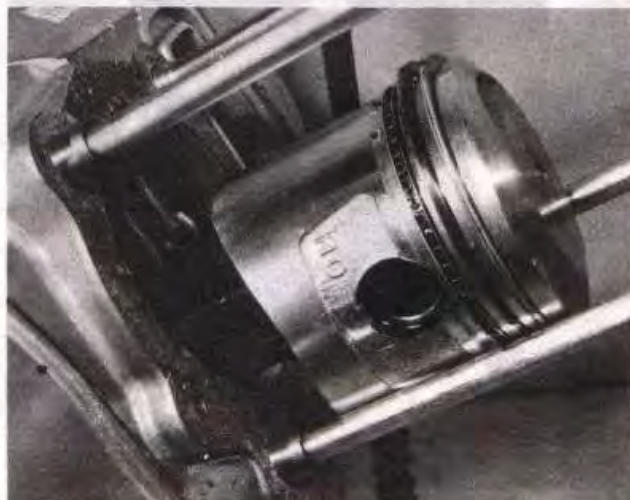
47.3 Refit the piston using NEW circlips ensuring their correct engagement
