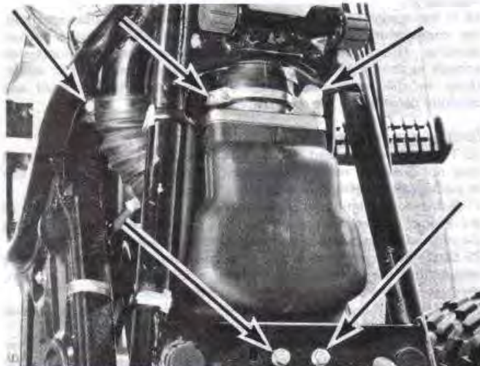
3.34 Remove the mounting bolts and loosen the clamp screws (arrows) to gain access to the air filter element
