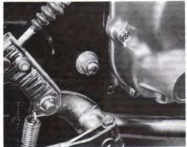
5.12b ... and the lower rear bolt to allow the engine to drop free, once the top bolts have been removed
