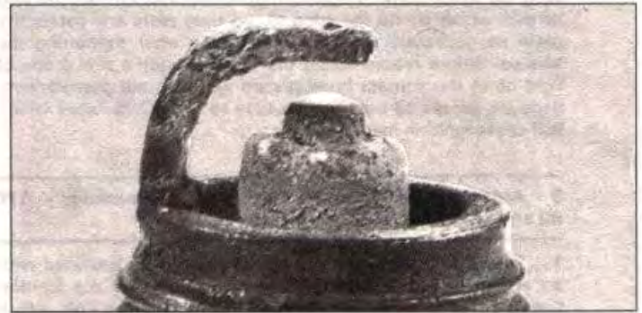
Worn plug - Worn electrodes will cause poor starting in damp or cold weather and will also waste fuel
