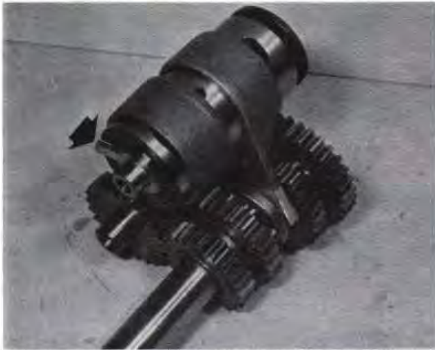
38.2 Do not omit the neutral switch contact (arrowed) during reassembly
