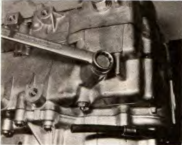
7.20 Remove bolt to allow cam chain tensioner components to be removed
