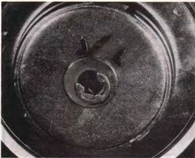
33.5a Remove the E-clip and washer and the plate
