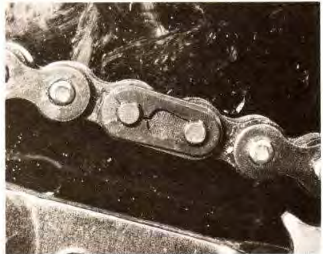
11.9 Make sure spring link is replaced correctly (this is the lower run of the chain)
