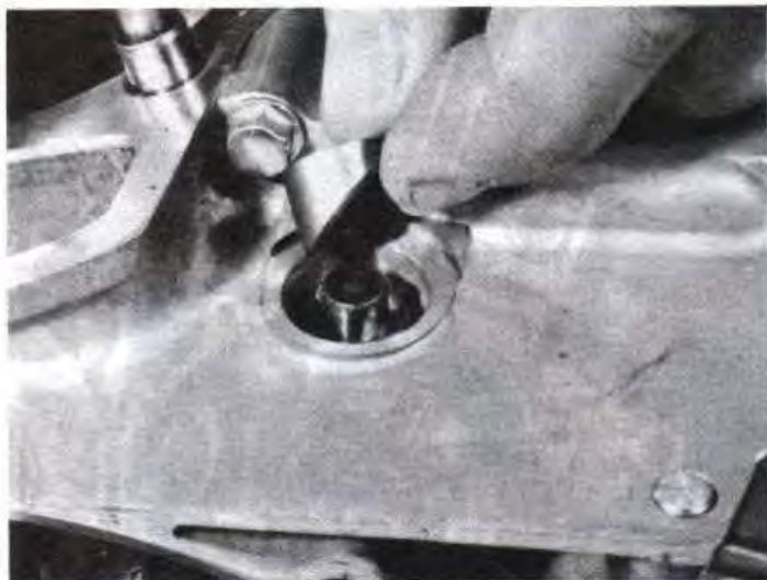
4.230a Installing the angled sleeves in the chain tensioner hole (they must slip over the tensioner plunger)
