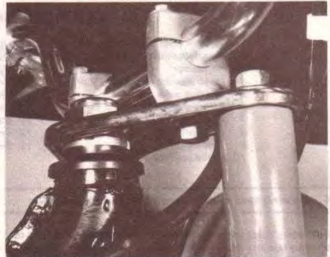
6.3b Replace the handlebars in the correct position; ensure all bolts are secure
