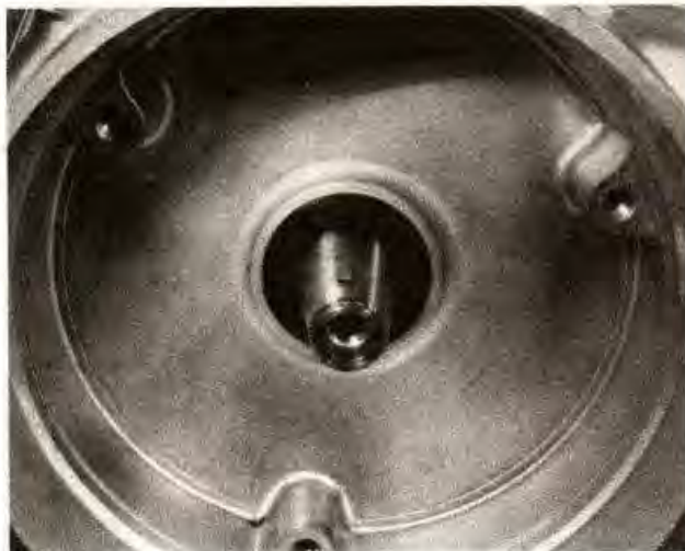
46.9a Install the Woodruff key in the crankshaft and notch before ...
