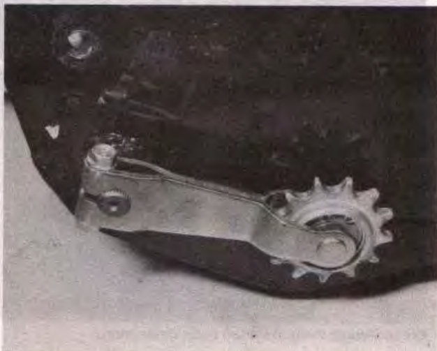
6.11 Remove the pinch bolt to slide the chain tensioner off the splined shaft.
