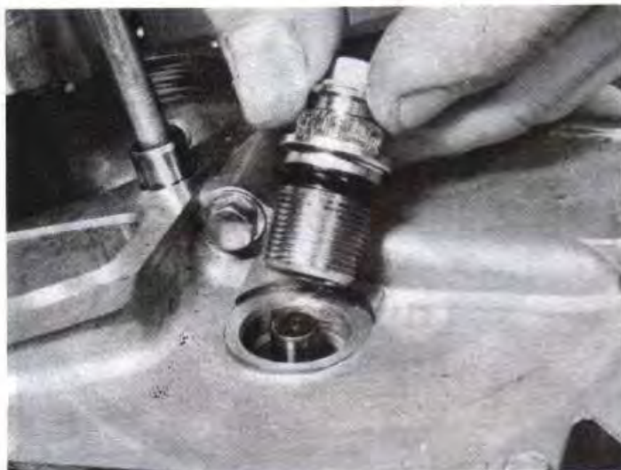
4.230b After checking the condition of the O-ring, screw in the adjuster bolt
