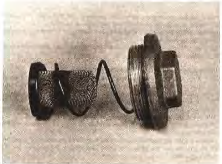
3.5 Be sure to install the oil filter screen, spring and cap exactly as shown
