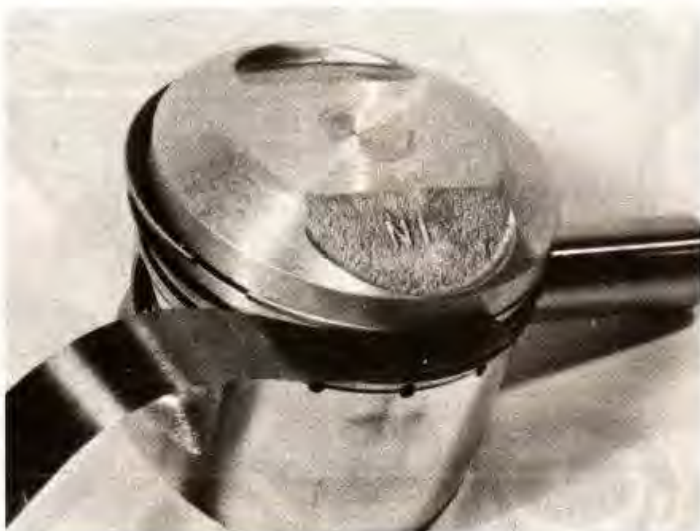
4.103 Measuring piston ring-to-groove clearance with a feeler gauge
