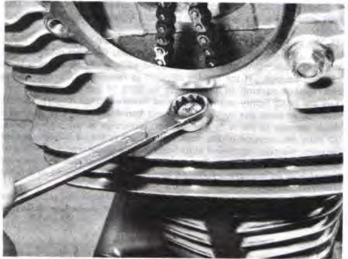
4.30a Before the cylinder head can be separated from the barrel, remove the bolt from the left side of the cylinder head
