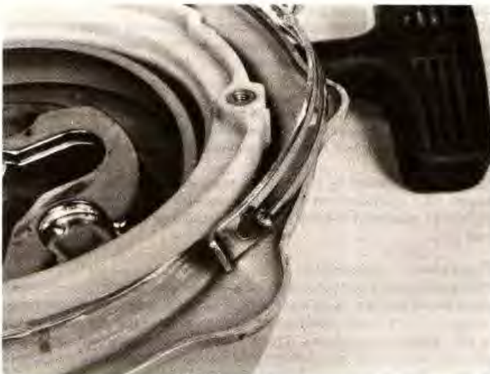
4.178a Installing the compression release slide onto the cable
