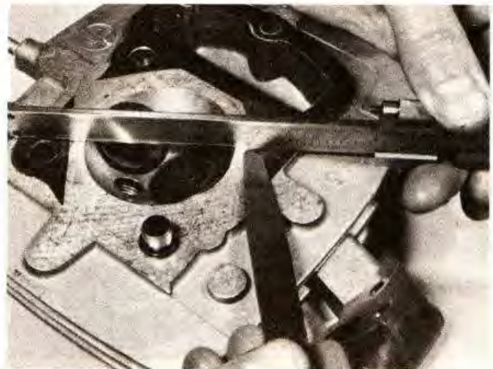
4.128 Checking the cylinder head gasket mating surface for warpage
