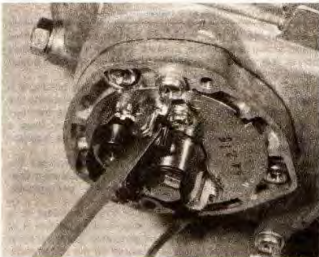
4.4 Check points gap in the fully open position using a feeler gauge (ATC 90/110)
