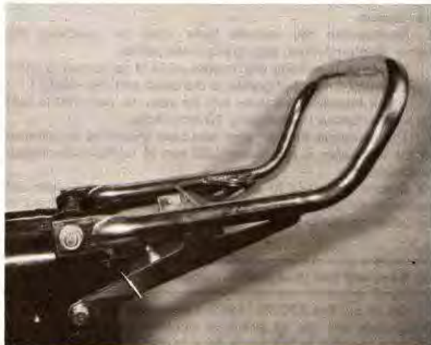
10.3 Rear grab handle secured by these nuts and mounting bolts
