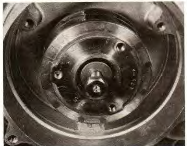
46.9b ... refitting the rotor and securing bolt (ATC 90/110)
