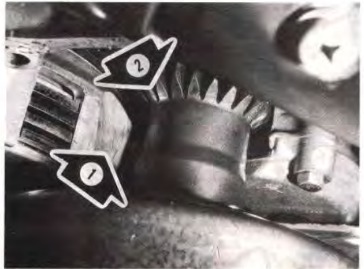
4.57 Align the cutout in the manual clutch housing (1) with the drive gear (2) and the centrifugal clutch drum can be removed from the crankshaft
