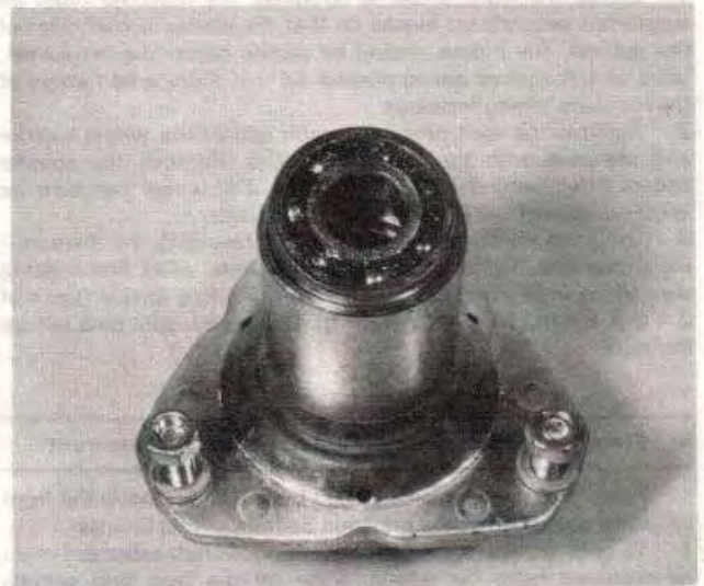
4.5a ... the bearings are now free to be tapped out ...
