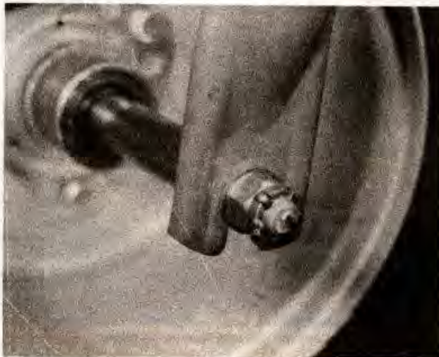
3.3 Fit a new split pin whenever the wheel is removed and replaced
