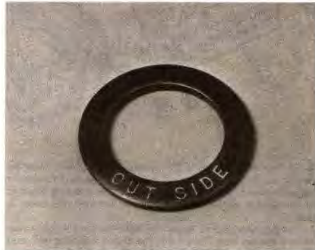
42.1a Note the marking on the Belville washer (ATC 110) ...
