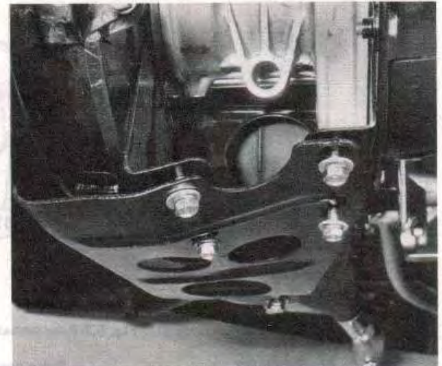
6.25a Refit the four 6 mm bolts at the rear end, and ...
