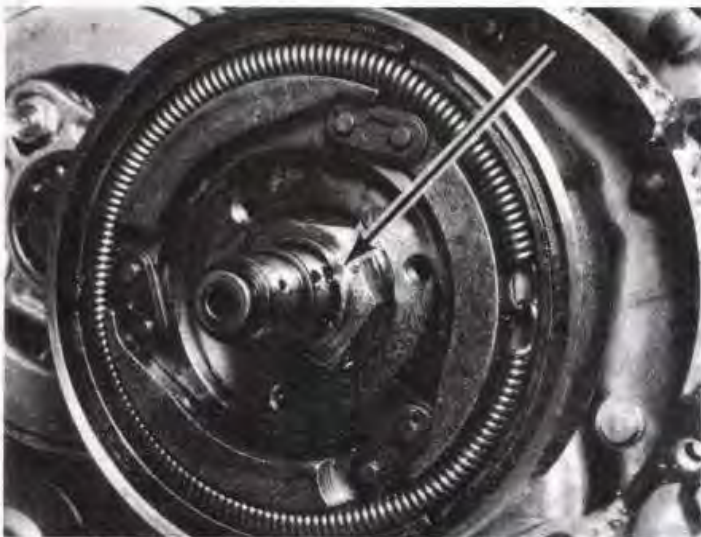
4.55 Pry the staked portion of the nut flange (arrow) out of the hole before loosening the nut
