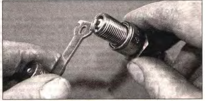
Electrode gap adjustment - bend the side electrode using the correct tool
