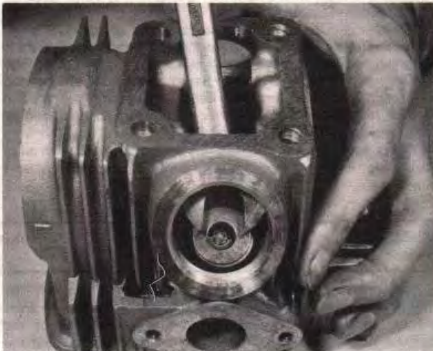
25.12e ... compress the springs to allow first one collet and ...
