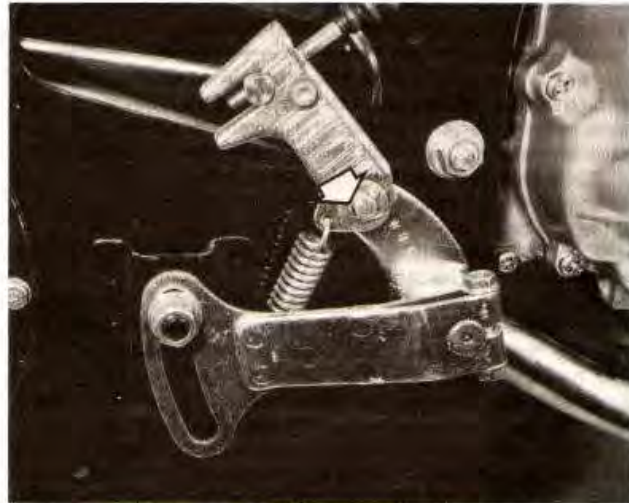
9.1 Ensure split pin (arrowed) is always fitted and return spring is in good condition
