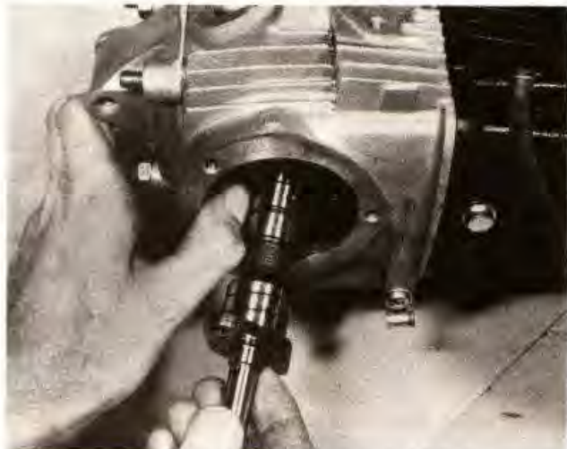
49.1 With the cylinder head and cover refitted, slide the camshaft into position (ATC 90/110)
