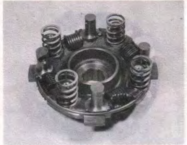
32.10 Examine all the springs thoroughly, especially the four main springs
