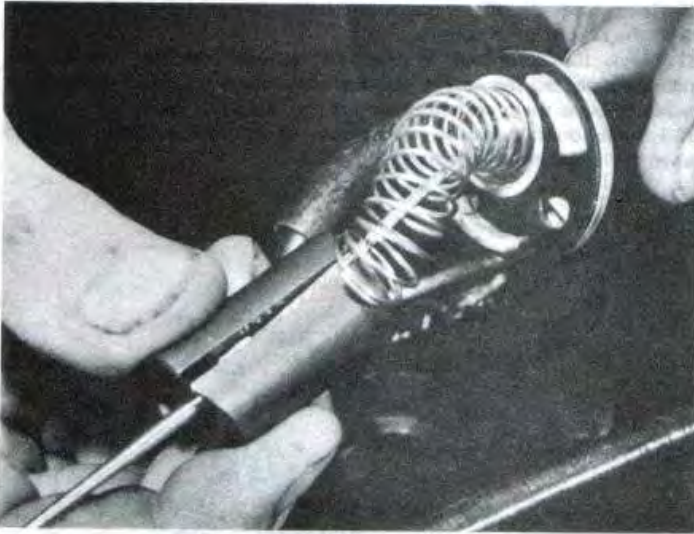
5.5 Disconnecting the slide/needle assembly from the throttle cable
