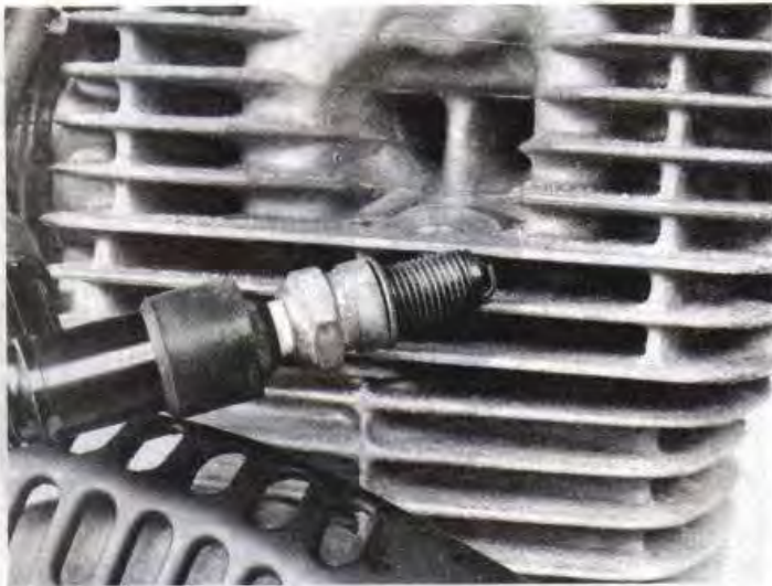
6.3 Checking for spark at the plug electrodes
