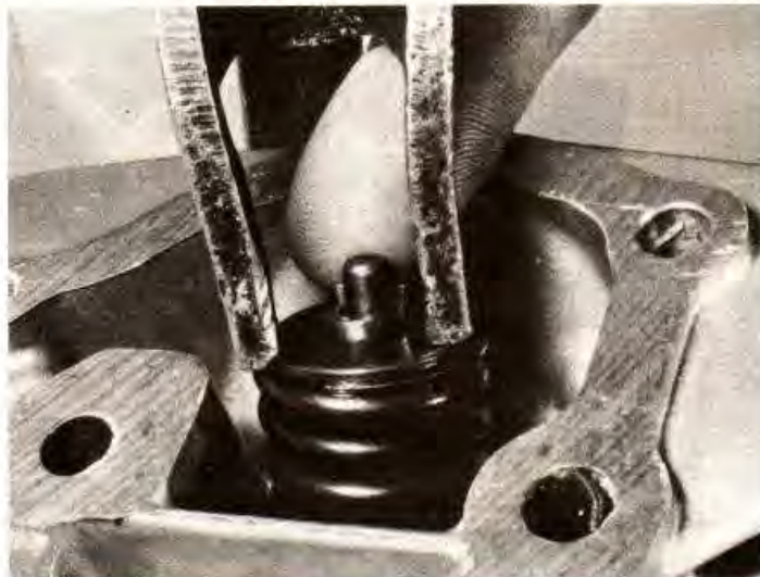
4.115 Removing the valve keepers with a valve spring compressor
