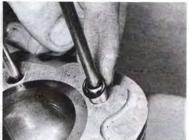
4.247 Positioning the O-ring over the dowel pin on the right rear cylinder stud
