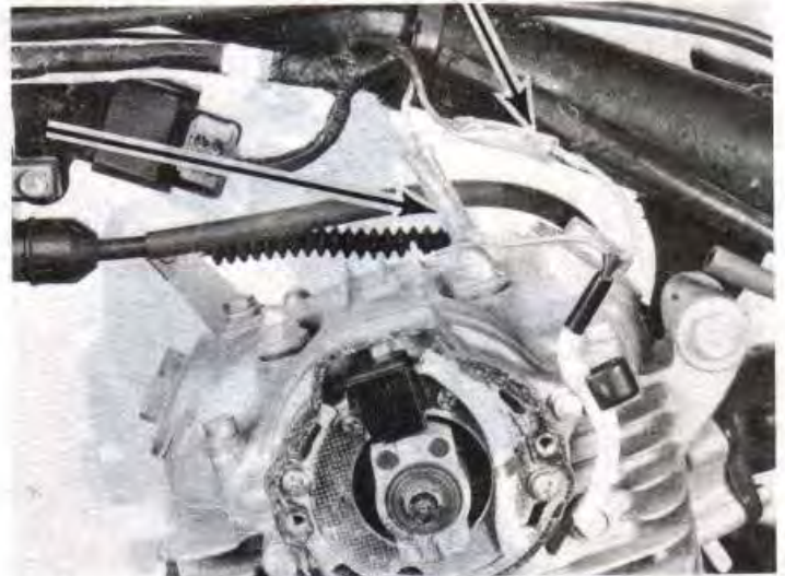
6.10 To check the pulser generator, unplug the wire leads (arrows) and measure the resistance between the wires coming out of the pulser coil
