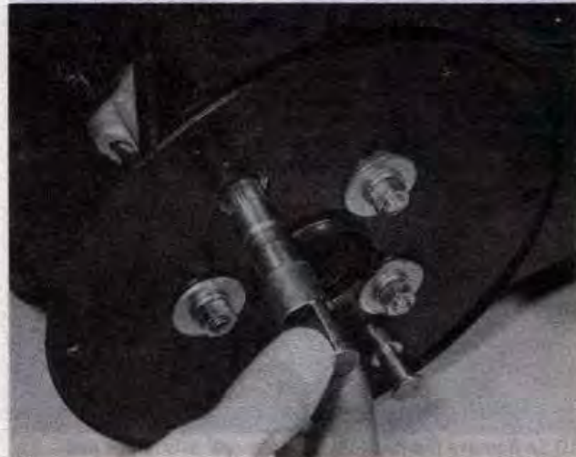
9.9a Note punch marks on brake operating arm and cam splined end, these should align ...
