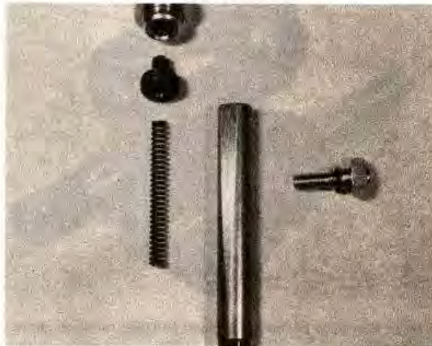
27.1b General view of cam chain tensioner components
