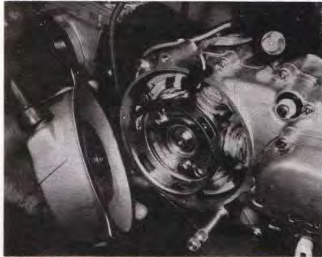
46.11 Refit the starter pulley, then the recoil starter and cover
