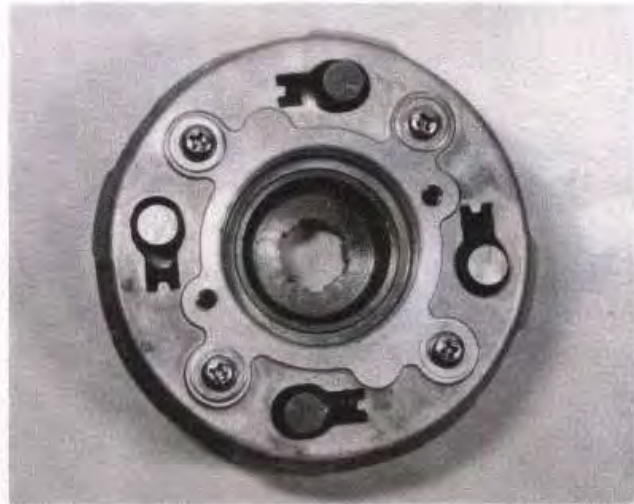
32.5 Remove the four screws to release the drive plate and springs
