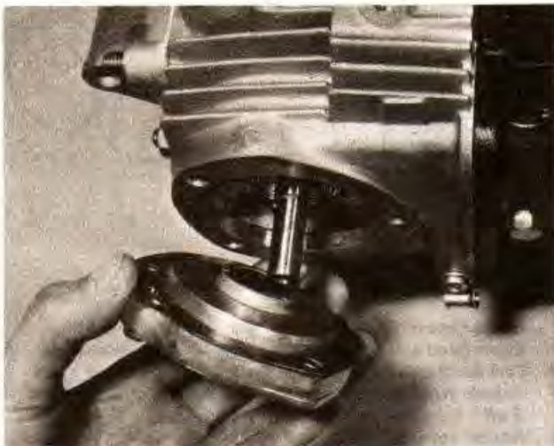
7.16 Detach contact breaker outer casing and gasket
