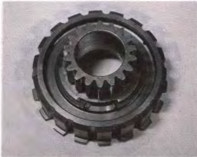
32.6a Remove the circlip from the clutch centre and ...
