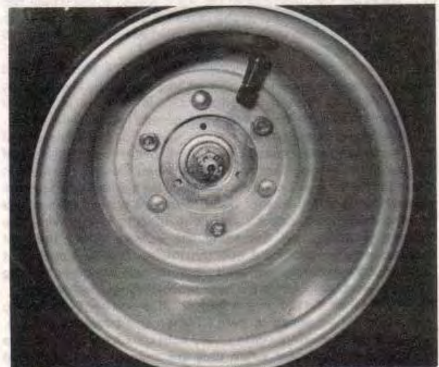
5.4 Removal of the three outward facing nuts allows wheel to be detached
