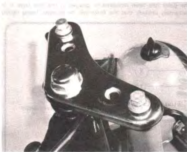
2.10a Slacken and remove the two top yoke bolts and ...
