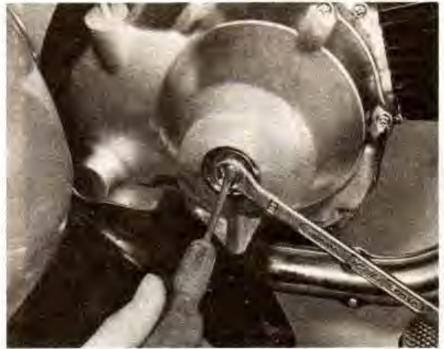
Set clutch adjustment with this adjuster and locknut
