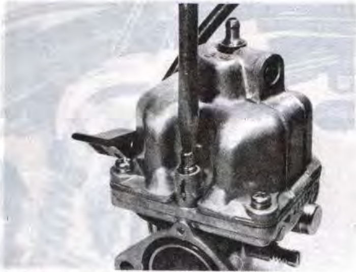
5.18 Removing the pilot screw from the carburetor body
