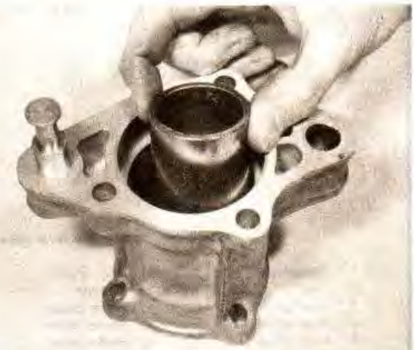
7.5c Large diameter hollow central spacer must be replaced upon reassembly
