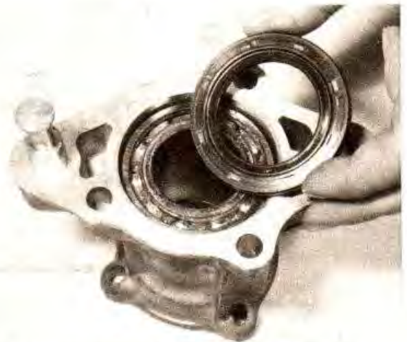
7.5a Renew oil seals if existing ones damaged in any way
