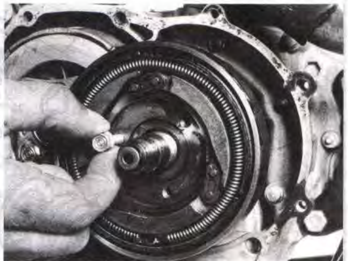
4.56 An oil filter cover bolt can be used to pull the centrifugal clutch weight assembly off the crankshaft
