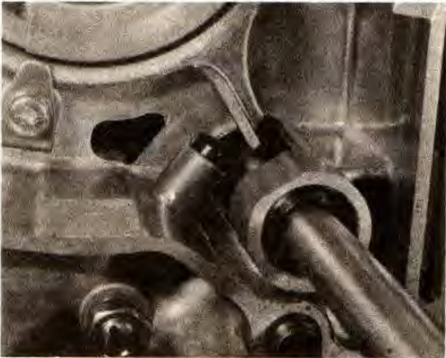
27.1a Check operation of cam chain tensioner pushrod and spring
