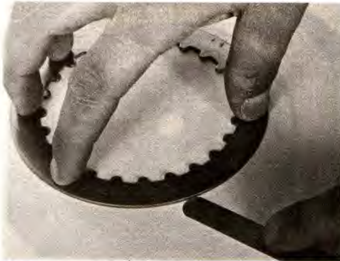
4.153 Checking a clutch plain plate for warpage
