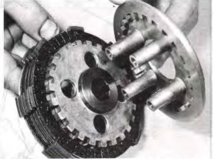
4.215 Assembling the clutch (note that the friction plate tabs are aligned in rows)
