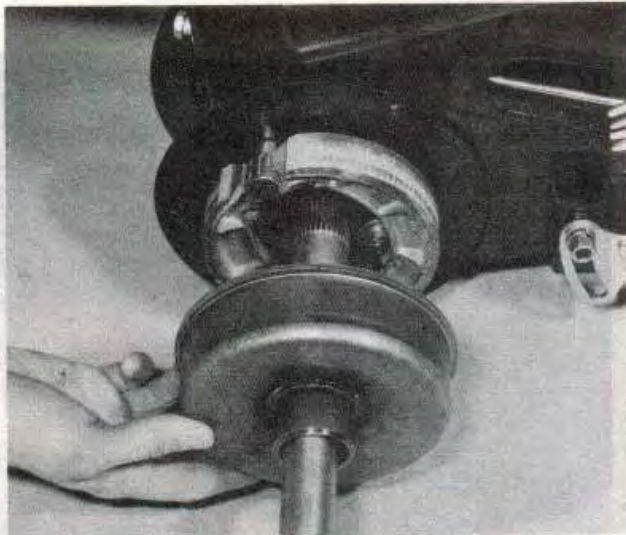
6.16c ... then the brake drum, leaving the shoes in situ
