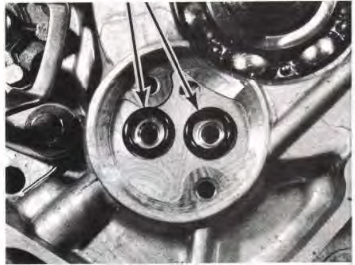
4.206 Be sure to install the O-rings (arrows) before attaching the oil pump to the crankcase
