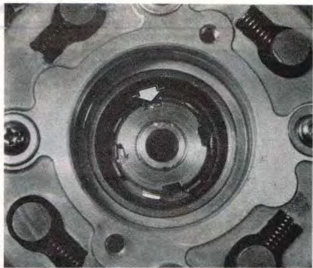
42.4c ... refitting pegged retaining nut and bending one tab into an appropriate slot in the nut (arrowed)
