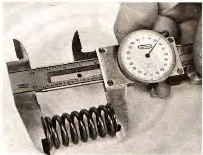
4.154 Measuring the clutch spring free length with dial calipers
