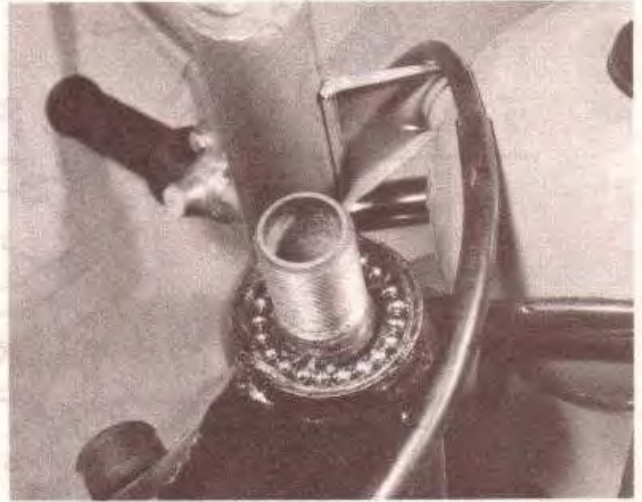
4.3 ... cup and cones of each bearing carefully
