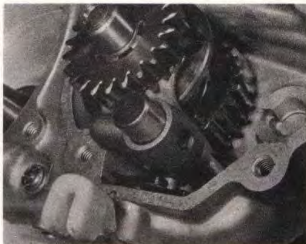
45.1b ... the selector fork and rod are fitted exactly right
