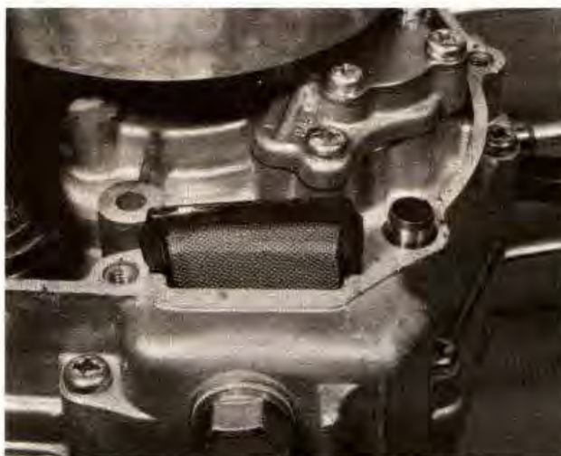
16.3 Remove gauze oil filter from crankcase slot for cleaning
