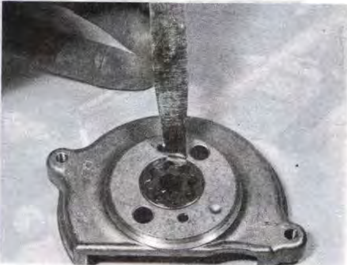
5.39a Checking the outer rotor-to-pump body clearance with a feeler gauge
