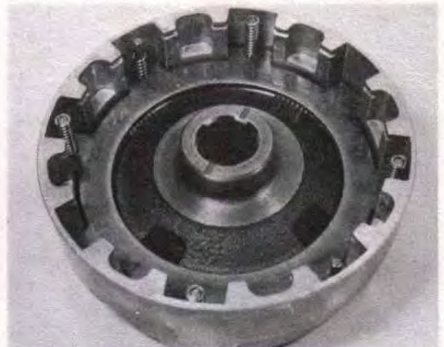
32.16 Note fitting of small springs on base-plate pins
