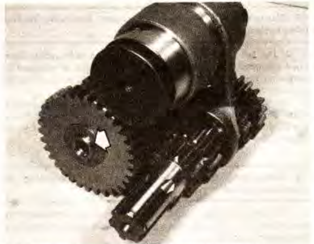
17.3 Do not misplace shim on outer pinion (arrowed)
