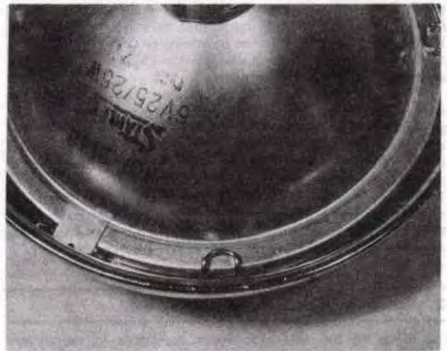
4.3b ... the four W-shaped securing clips
