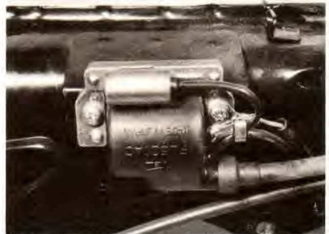
23.3 The coil and condenser are mounted together on the frame (ATC 90/110)
