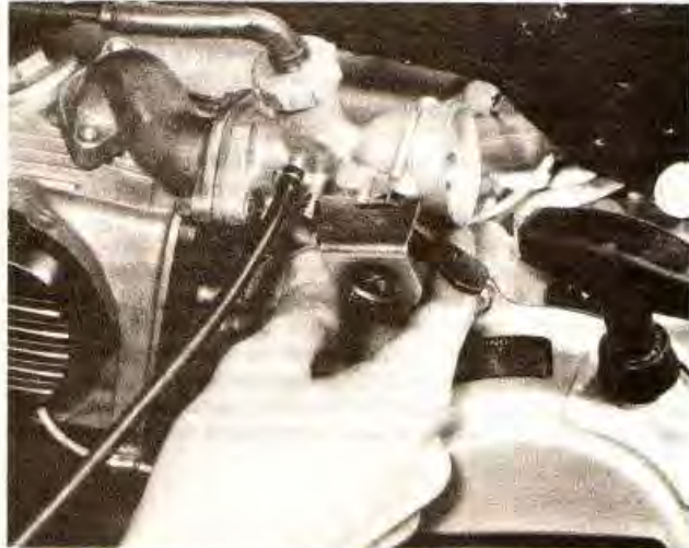
5.5 Lift away carburettor complete with manifold and overflow pipe
