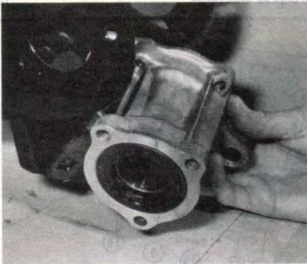
6.21 ... then remove the axle central hub
