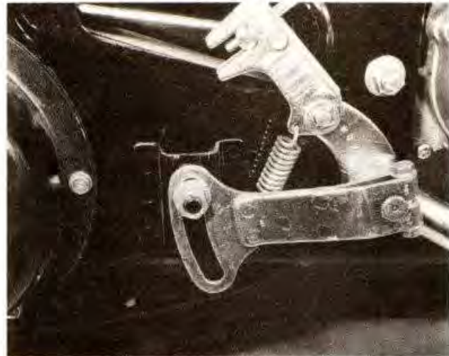
Slacken the locking nut (ATC 90/110) on chain tensioner to enable arm to move upwards to adjust chain
