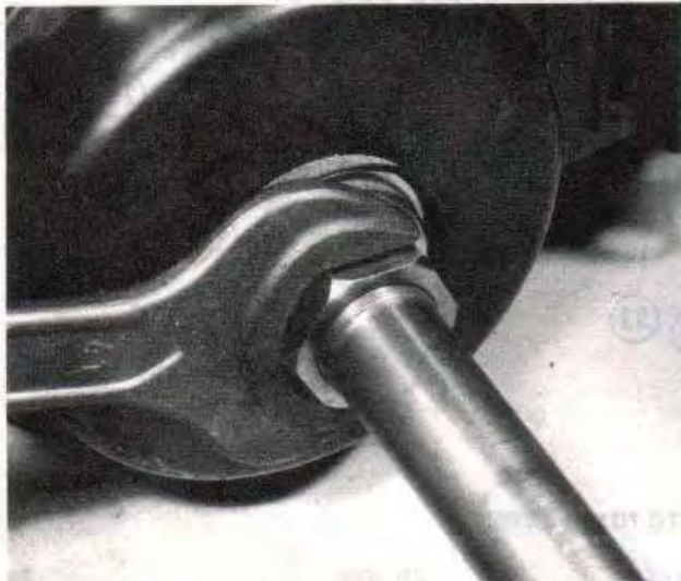
6.24b ... replacing and tightening the large brake drum nuts
