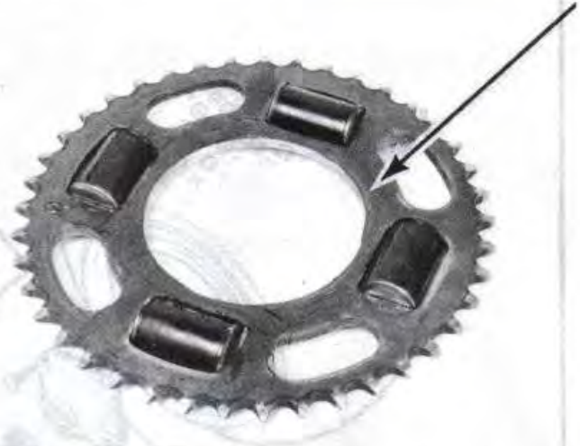
8.22 Apply a thin layer of grease to the sides of the sprocket (arrow) before assembling the damper plates
