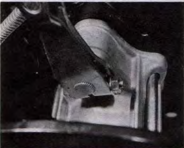
9.9b ... before replacing the operating rod and adjuster nut
