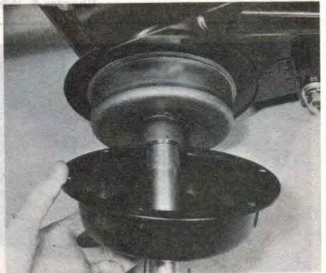
6.16b Detach the brake drum outer cover and ...
