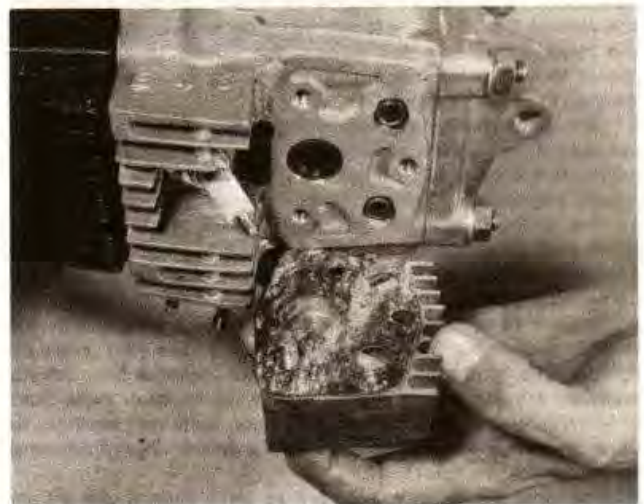
7.19 Detach the right hand side head cover and gasket
