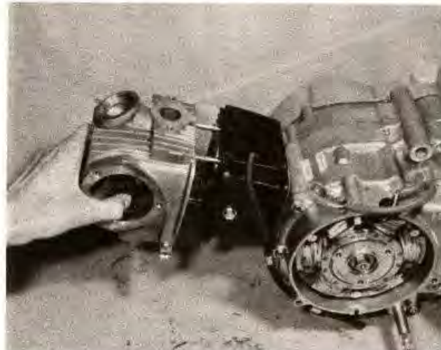
7.23 Lift the cylinder head away from the barrel
