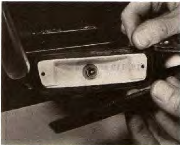
5.1 Rear lamp lens is retained by two screws
