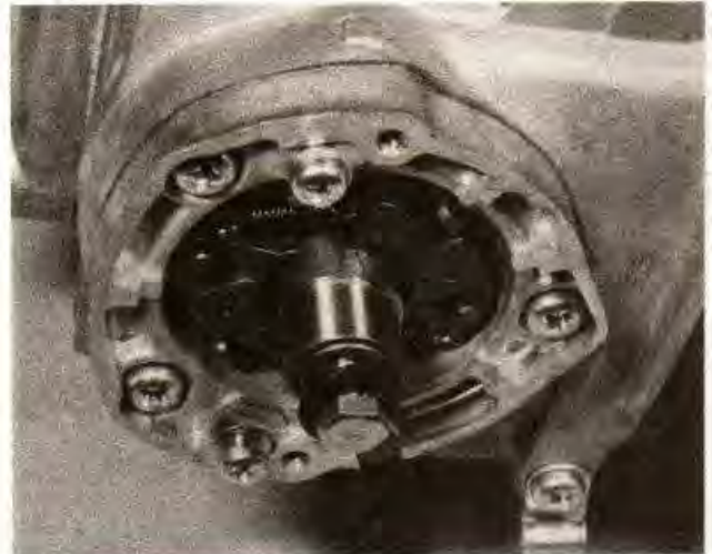
7.15 Remove hexagon head bolt to withdraw ATU from camshaft
