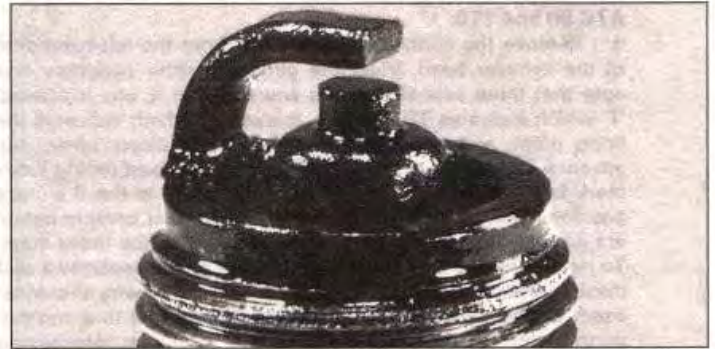
Oil fouling - Wet oily deposits leading to misfire and weak spark. Caused by oil leakage past piston rings or valve guides (4-stroke engine), or excess lubricant (2-stroke engine)
