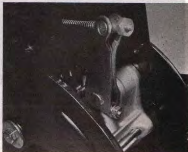
6.14a Disconnect the brake cable from the arm at the top and ...
