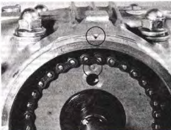
4.260 The O mark on the sprocket must be aligned with the index mark (circled) on the cylinder head cover before installing the sprocket mounting bolts
