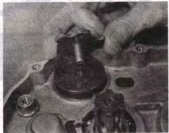
41.4 Refit the four small pins and secure them with the index plate
