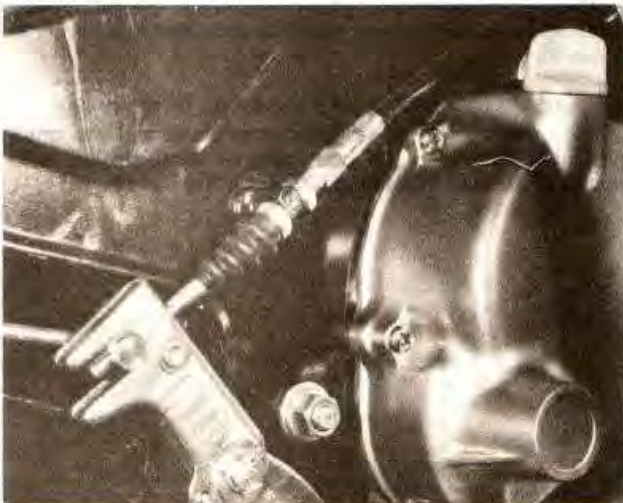
Use the cable adjuster nuts to make brake lever adjustment (ATC 110 shown)
