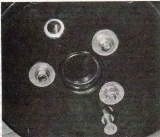
6.19a Undo these nuts to release the brake drum base plate and ...
