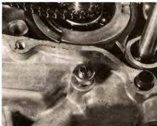
Adjust cam chain tension firstly with this adjuster and locknut and then ...
