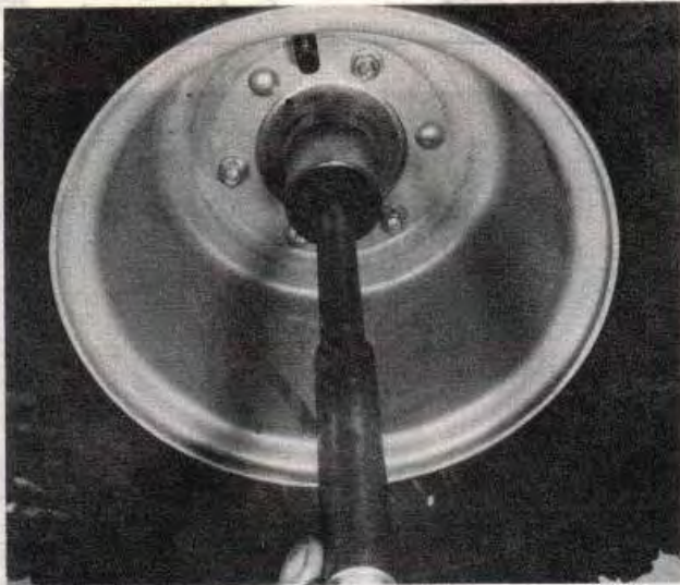
4.2a Remove wheel spindle and spacers to allow ...
