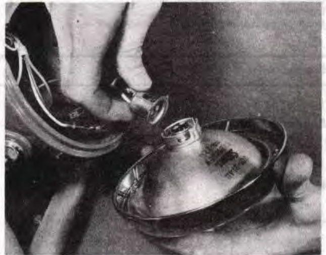
4.2 Twist and pull out the bulb holder
