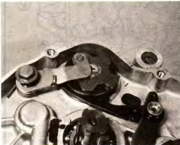
12.1 Remove shouldered bolt and index arm and spring
