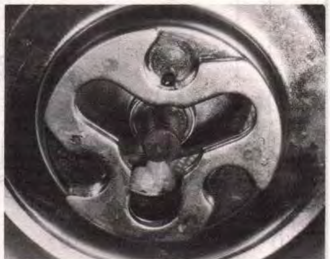
33.5d ... removing the weights for examination
