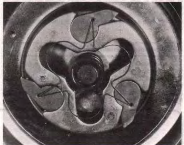
33.5b Detach the wire springs and central spring and washer
