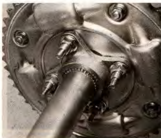
10.11a The outer four nuts secure the sprocket and two backing plates assembly
