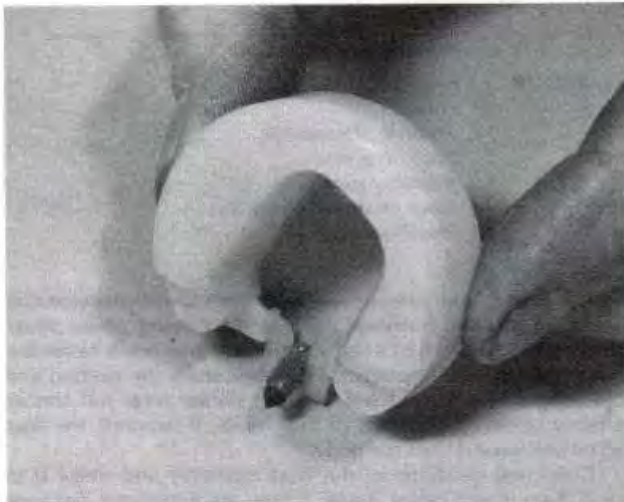
8.3c Take care not to lose the small float needle
