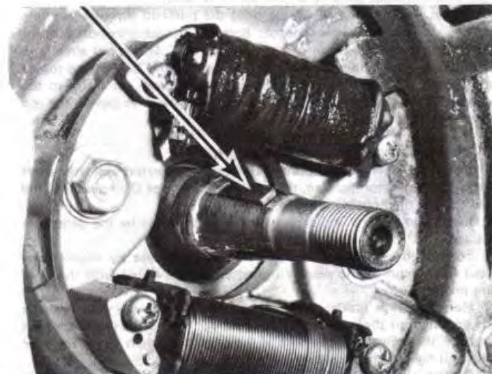
4.235 Make sure the key is in place before sliding the rotor onto the crankshaft
