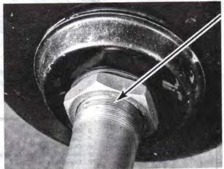
8.25b After the inner nut is installed, apply thread locking compound to the threads (arrow), then install and tighten the outer nut
