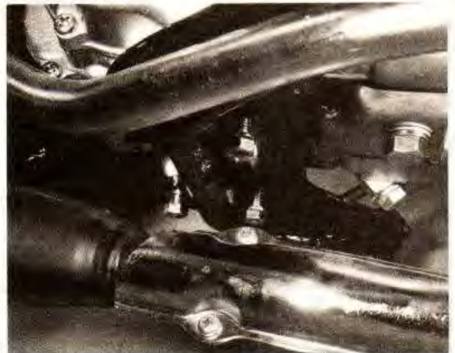
8.1 The footrest bracket is secured by four bolts under the engine
