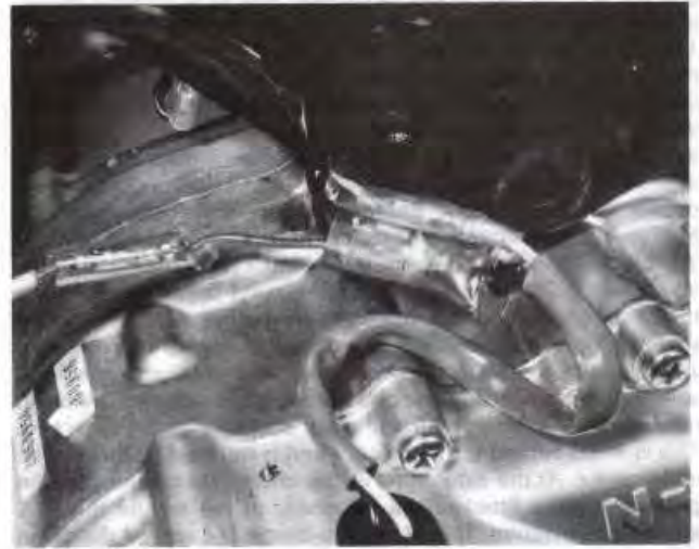
5.10 Disconnect all wires at the snap connectors
