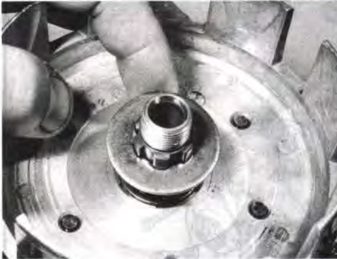
4.214 Be sure to install the thrust washer before sliding the clutch assembly onto the shaft
