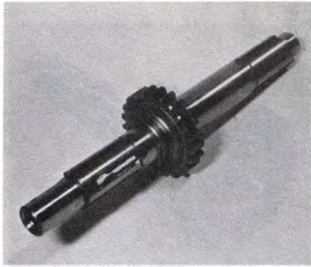
29.6d To the transmission layshaft fit ...
