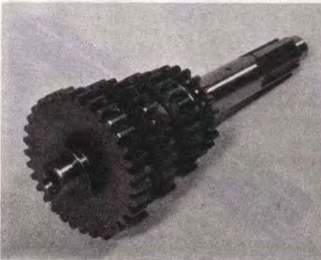
29.6i Finally, refit end shim to layshaft
