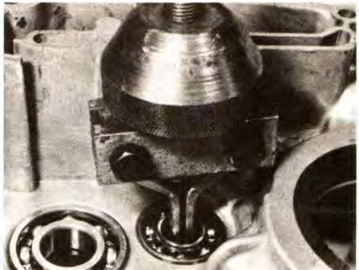
4.89 Using a slide hammer-type puller to remove a transmission bearing
