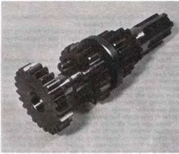
29.6c ... the mainshaft top gear pinion (24T)
