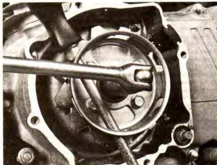
4.42 Loosening the AC generator rotor mounting nut
