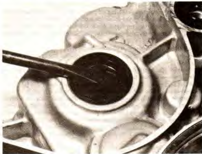
4.85a Oil seals can be pried out of place with a large screwdriver
