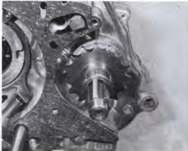
15.2 Slide off the primary final drive sprocket
