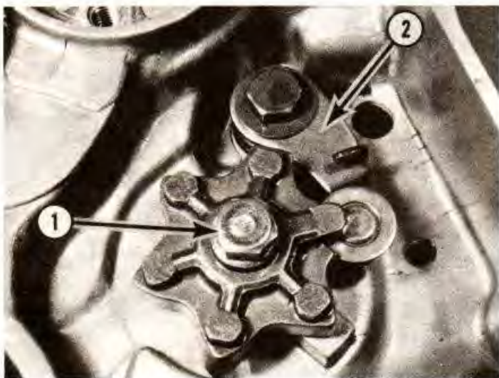
4.69 Loosen, but do not remove, the bolt in the center of the drum stopper plate (1), then remove the stopper arm (2)
