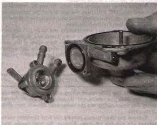
4.7 ... check the condition of tap and chamber sealing rings
