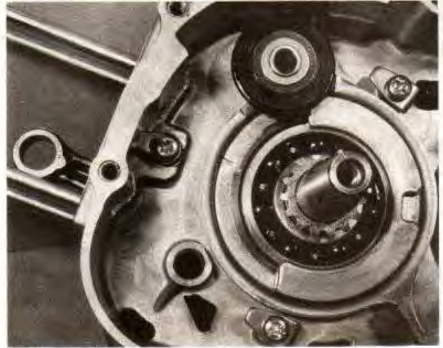
43.2a Refit the cam chain tensioner ring and ...
