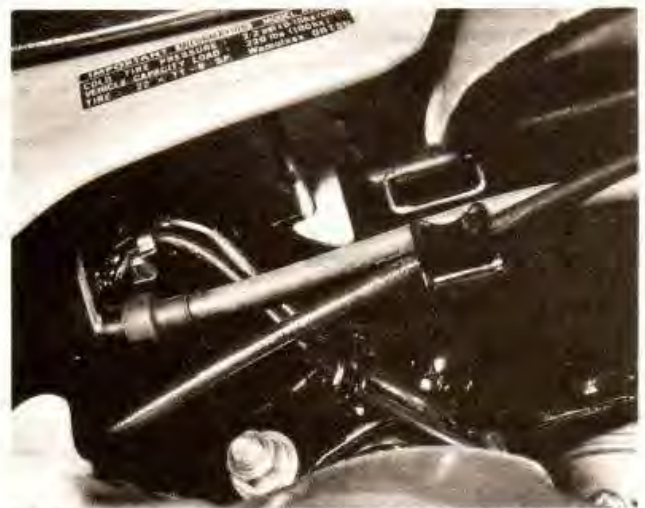
5.3 Operate lever to release bodywork and detach tank retaining strap
