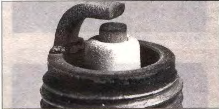
Normal condition - A brown, tan or grey firing end indicates that the engine is in good condition and that the plug type is correct
