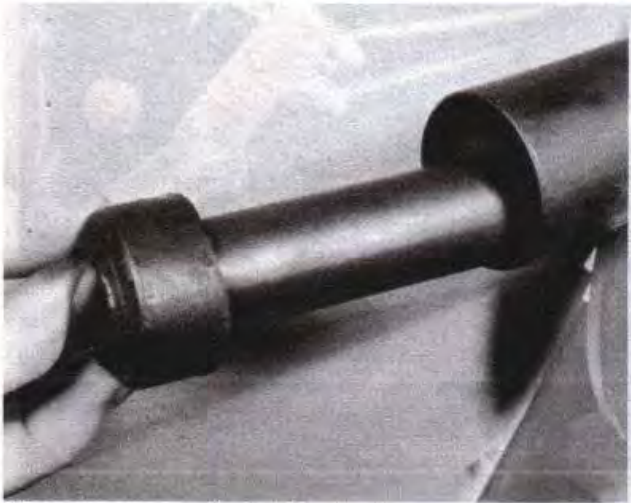
The spark arrester pulls clear for cleaning
