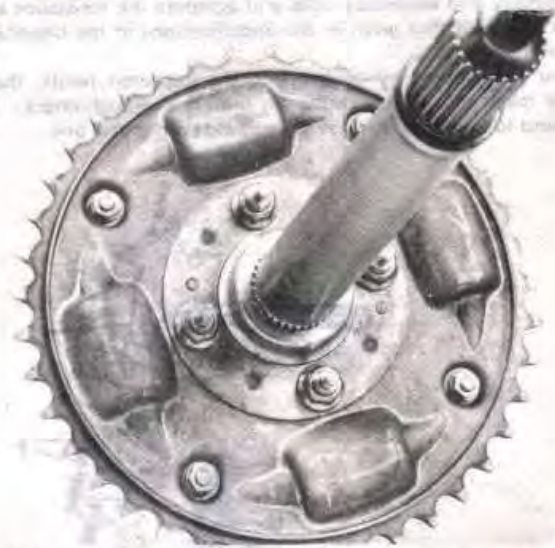
8.15 The sprocket/damper assembly bolts must be removed to separate the sprocket from the axle
