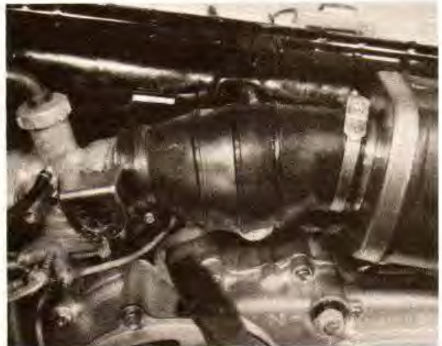
6.5 Detach rubber intake hose from rear of carburettor
