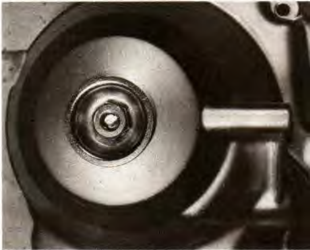
42.11b ... the clutch adjusting bolt and locknut will probably need slackening
