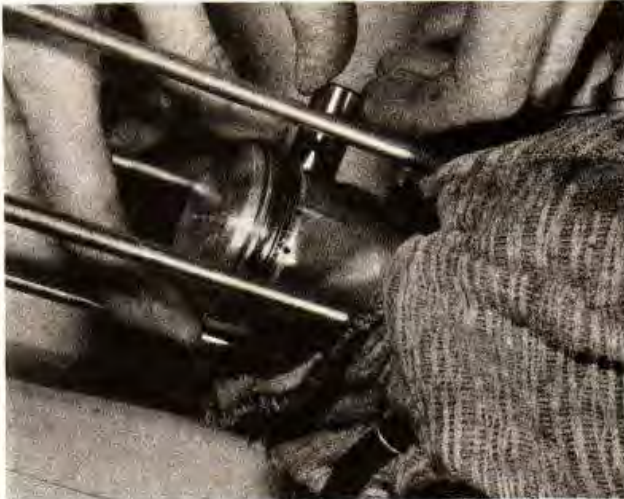
8.3 Slide out the gudgeon pin, and discard the used circlips
