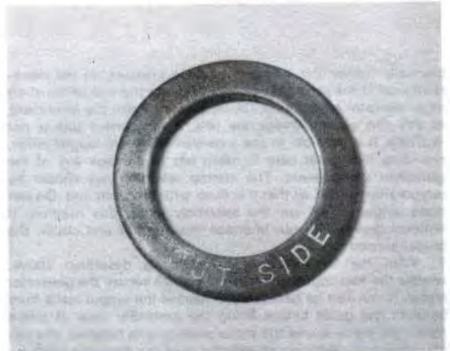
10.9 Note the marking 'OUTSIDE' on the Belville washer
