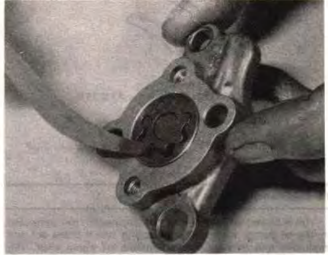
18.4b ... inner rotor/outer rotor tip clearance
