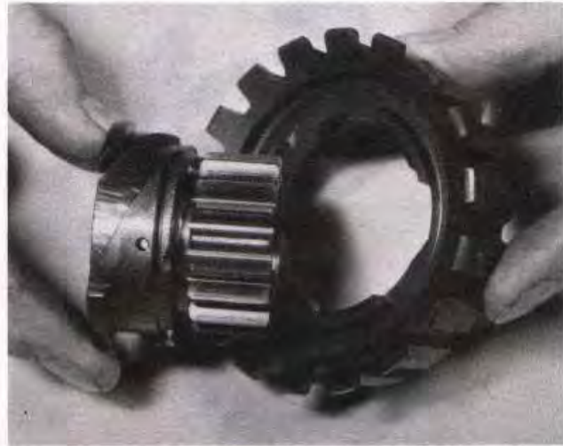
32.6b ... separate the centre and the primary drive gear pinion
