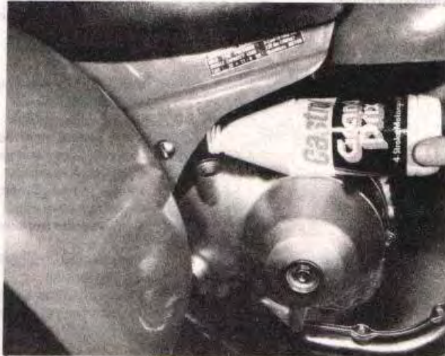
52.6 Refill with correct oil to full mark on dipstick
