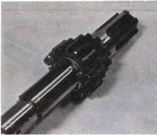
29.6a Slide the mainshaft second gear pinion (18T), onto the mainshaft and ...
