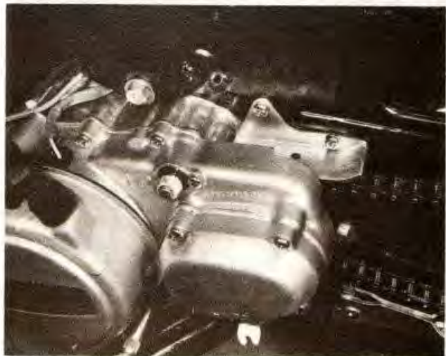
5.7 Remove chain guide plate (ATC 90 post K2 and ATC 110) to facilitate chain removal
