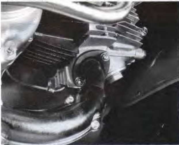
5.9 Remove the two exhaust pipe flange retaining nuts
