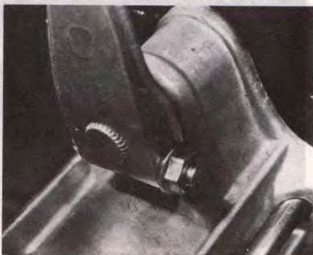
6.14b ... remove the bolt at the bottom of the arm
