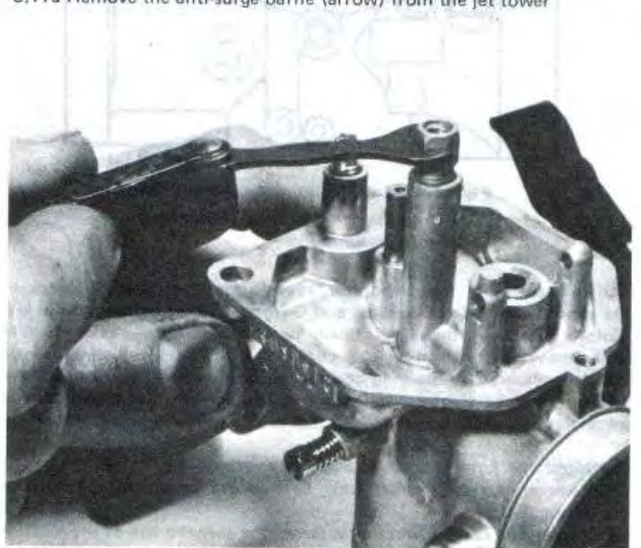
5.17c ...then remove the needle jet holder with a small wrench
