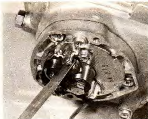
Contact breaker gap is measured with feeler gauge (ATC 110 shown)
