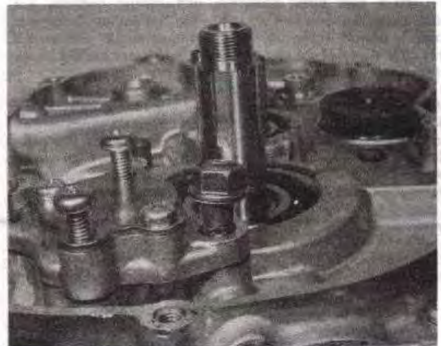
41.1b ... refit the screws and bolt (ATC 90/110) and tighten fully
