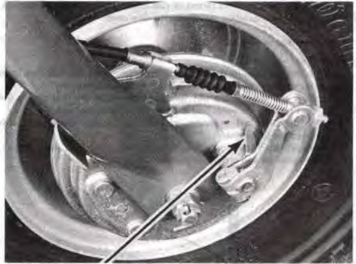
3.50 The brake shoe wear indicator (arrow) simplifies brake shoe inspection procedures
