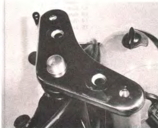
2.10c ... to allow the top yoke to be lifted away
