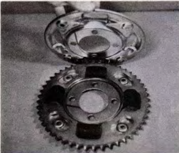
10.6a Lift off the outer backing plate to gain access to ...
