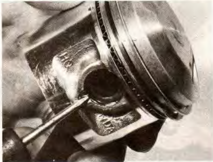
4.37 Prying a piston pin retaining circlip out of the piston
