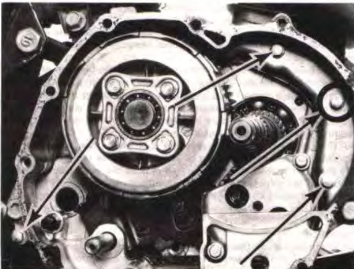
4.65 The crankcase spacer is attached to the crankcase with four bolts; make sure the longest bolt (circled) is returned to its original location
