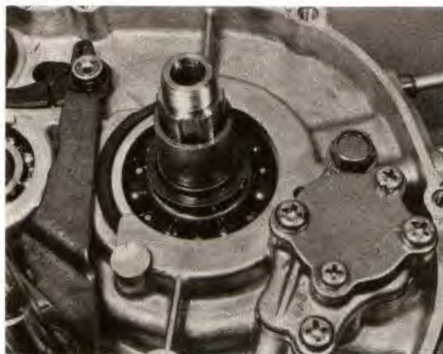
42.1c ... the double diameter spacer and clutch centre bush
