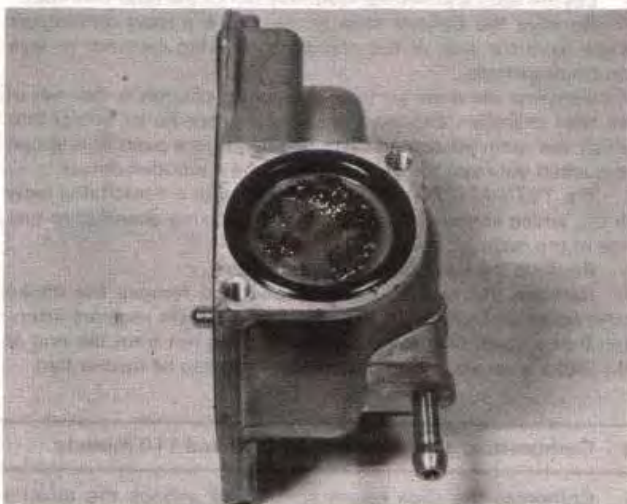
4.6 Clean the gauze in the float chamber side and ...
