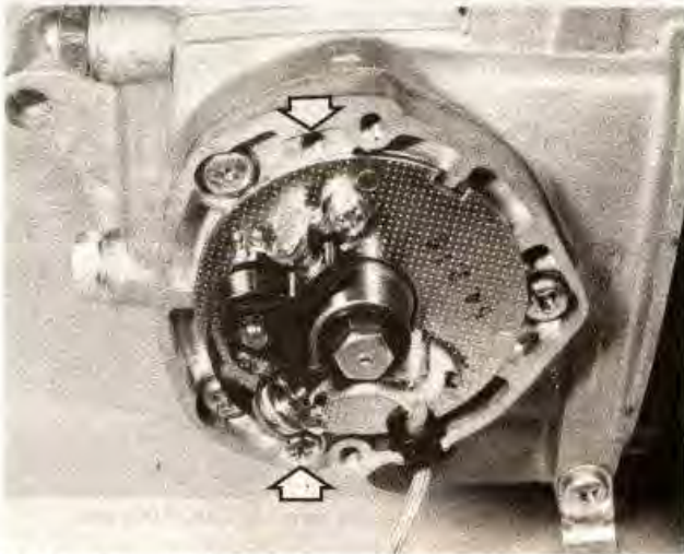
50.22 ... then refit the points assembly and secure it with the two screws (arrowed)
