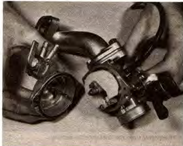
8.2 Separate the float chamber from the carburettor body
