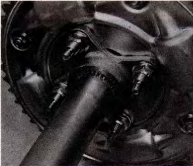
10.5a Remove the four nuts from the rear axle flange and ...
