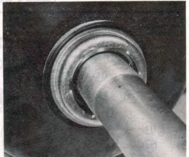
6.24a Do not omit the brake drum dust seal/washer before ...
