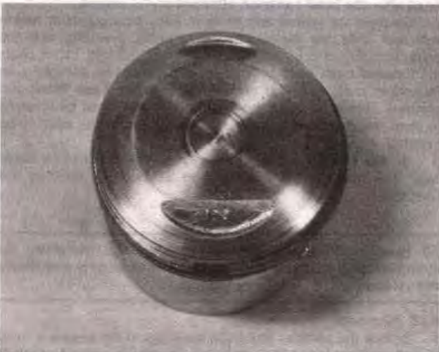
47.2 Cutout for inlet valve is marked appropriately (ATC 90/110)
