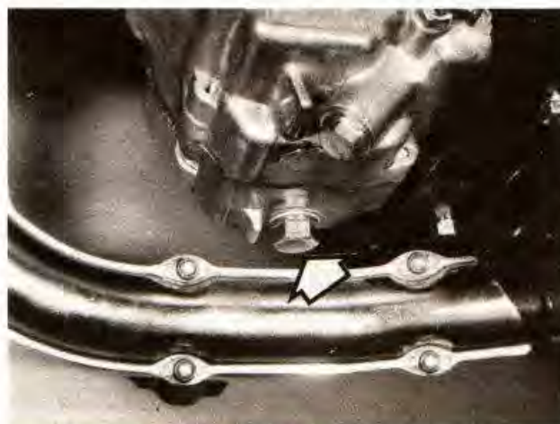
Remove drain plug (arrowed) and allow old oil to drain
