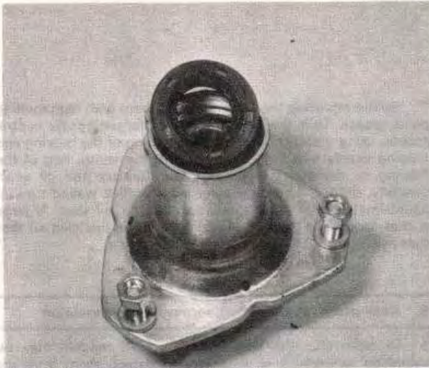
4.4 Prise out the oil seal carefully so that ...
