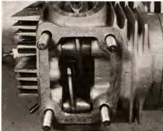
49.2 Exhaust rocker arm must be lowered to allow inlet rocker to be fitted
