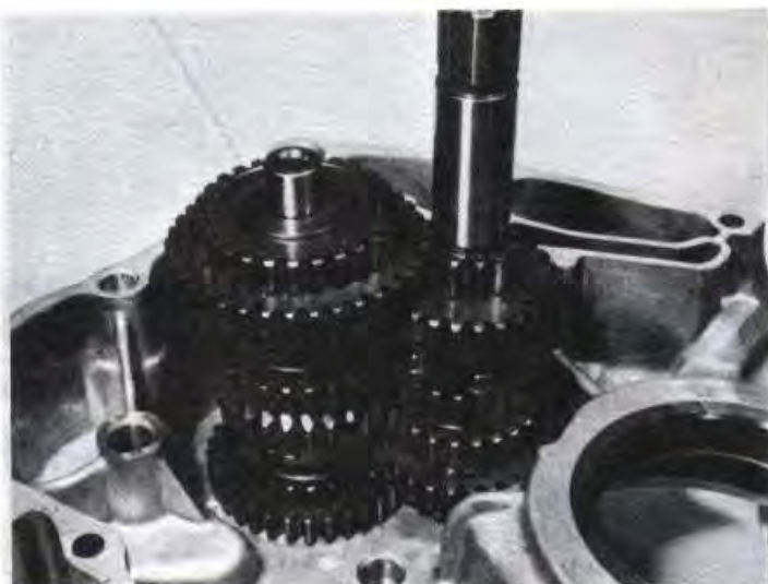
4,192 The built-up transmission shafts can be installed as a unit in the left crankcase half
