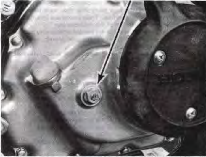
3.43 Clutch adjusting screw location
