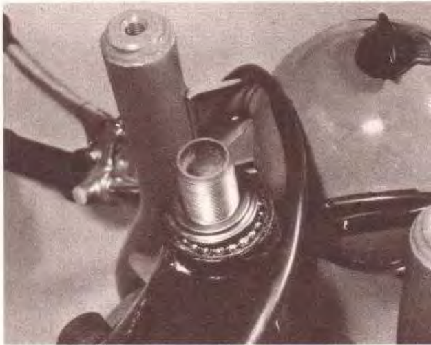
4.1 Note the gap which each race must have and examine the ...
