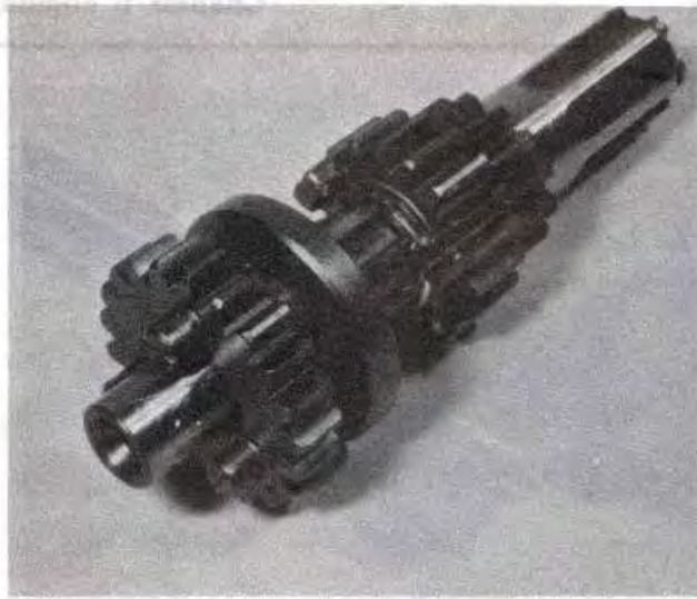
29.6b ... secure it with the splined washer and circlip. Then fit the mainshaft third gear pinion (21T) followed by ...
