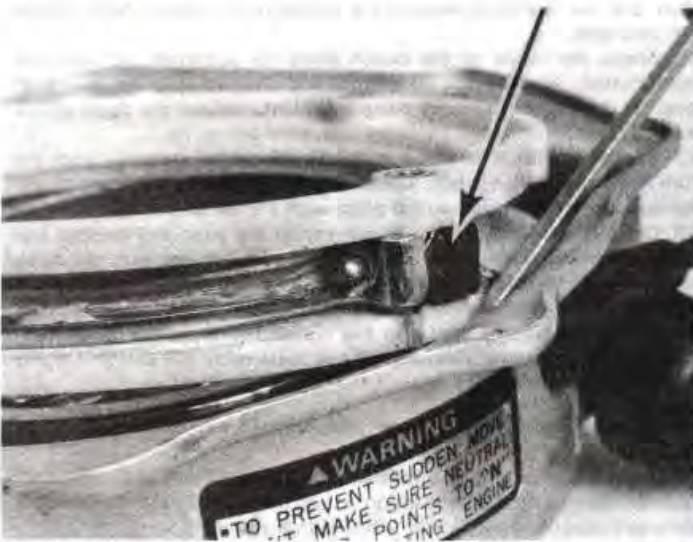
4.168 Pry up the nylon guide, then remove the rubber stop (arrow) and the cable
