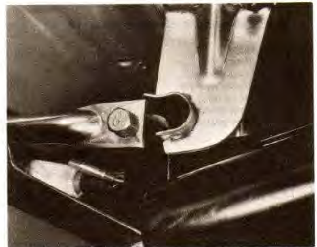
12.1b ... ensure rear of bodywork re-locates here upon refitting
