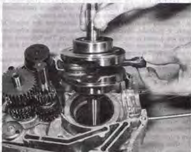
17.1 Crankshaft assembly lifts easily out of case
