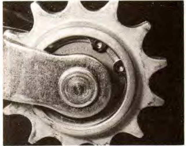
11.4b ... the tensioner toothed pulley wheel is contacting the chain. A circlip retains the toothed pulley wheel
