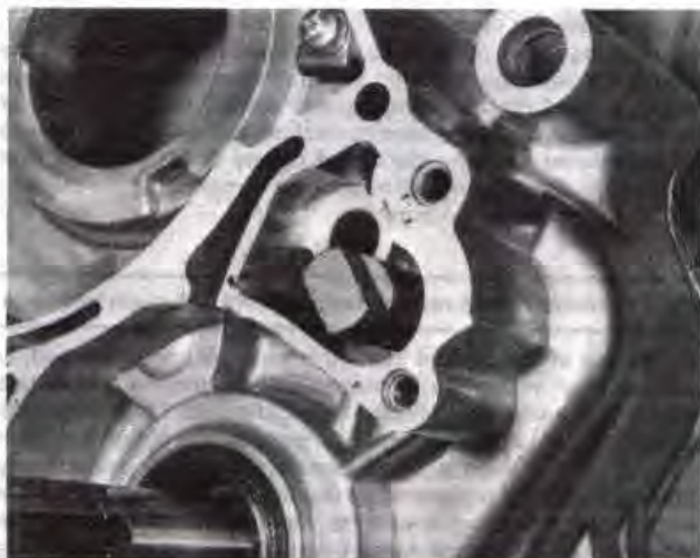
16.3 Remove the innermost section of the neutral indicator shaft before splitting crankcase halves
