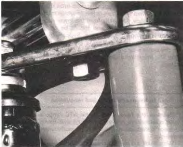
2.6a Slacken the handlebar clamp retaining bolts and ...
