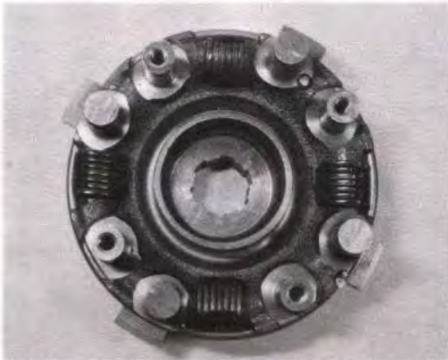
32.4 Remove the four bob-weights on the large clip behind the drive plate
