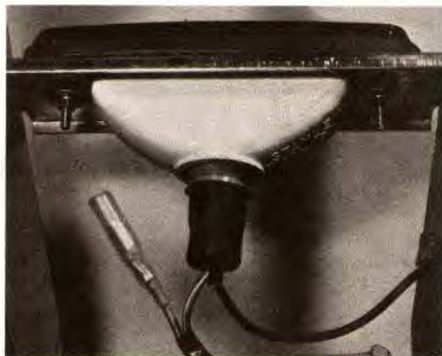
5.2 Bulb holder has rubber shroud behind holder
