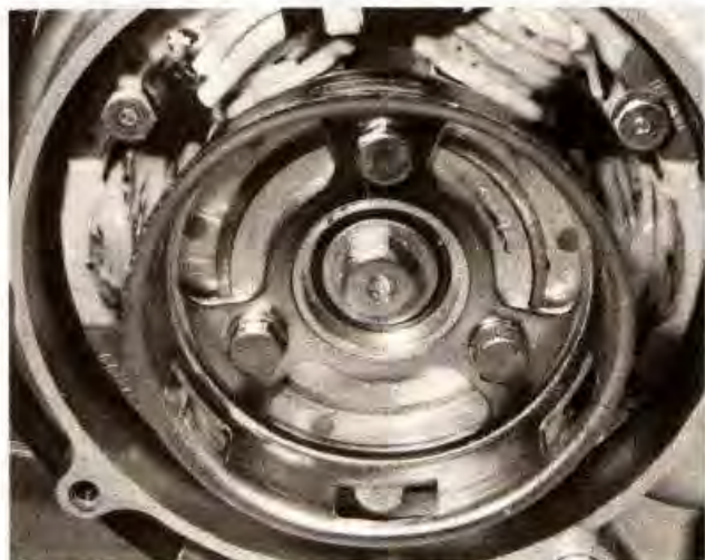
9.3 Remove the three (or four) bolts to detach the recoil starter pulley
