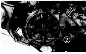
14. Remove the primary wire connector, remove the three 6 mm screws securing the stator and then remove the stator from the left crankcase cover.
