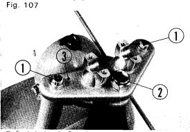
① Fork bolt ② Steering stem nut ③ Fork top bridge Fig. 108
