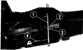
① Seat stopper ② 6 mm washer ③ 2 mm split pin ④ Cover set spring Fig. 89
