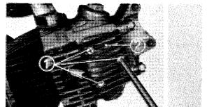
13. Remove the three 6 mm screws and remove the rocker arm side cover.
