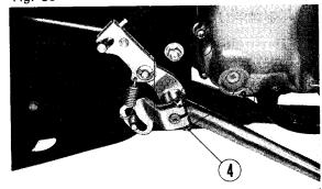
① Tensioner lock arm ② 6 mm bolt ③ 6 mm plain washers ④ 6 mm nut Fig. 86
