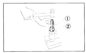
(1) Bearing driver handle(2) Oil seal driverFig. 31
