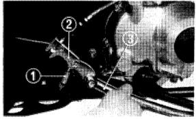
(1) Spring (2) Escape lever (3) Brake pedal Fig. 181
