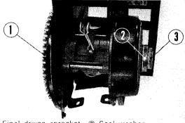
① Final driven sprocket ② Seal washer ③ Brake drum nut
