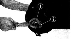
10. Apply grease on the tensioner shaft, and then insert it into the frame.
