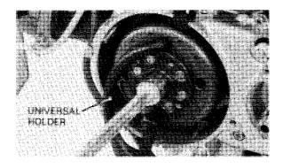
Remove the A.C. generator rotor with rotor puller No. 07933-001.
