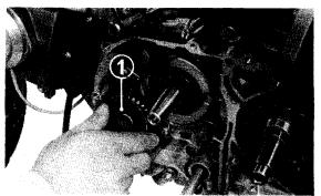
(1) Cam chain guide roller (2) Cam chain tensioner
