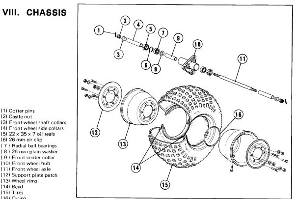
(4) Front wheel side collars (5) 22 x 35 x 7 oil seals (6) 26 mm cir clip (7) Radial ball bearings (8) 26 mm plain washer (9) Front center collar (10) Front wheel hub (11) Front wheel axle (12) Support plate patch (13) Wheel rims (14) Bead
