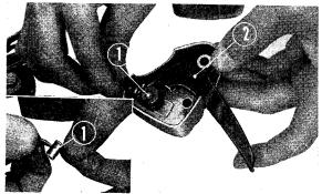
① Throttle cable end ② Throttle lever Fig. 67
