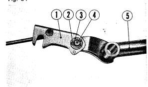
① Escape lever ② 2 mm split pin ③ 8 mm washer ④ Escape shaft ⑤ Brake pedal Fig. 85
