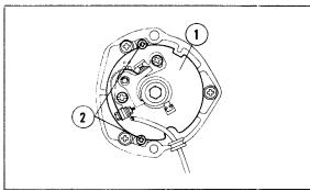
(1) Contact breaker base plate (2) Base plate locking screw
