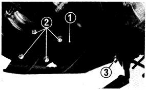
18. Remove the four 6 mm bolts securing the protector and loosen the one 8 mm bolt.
