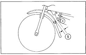
(1) Install the 16–21 mm (In the straight ahead position)
