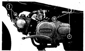
(1) 8 mm engine mounting bolts(2) 10 mm engine mounting bolts
