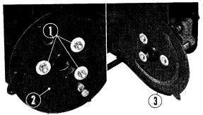
① 6 mm bolts ② Brake drum cover A
