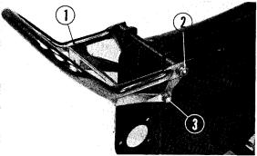
① Carry pipe ② 10 mm bolt ③ 8 mm bolt
