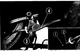
① Lock nut ② Adjuster nut ③ Brake lever clip ④ Front brake lever
