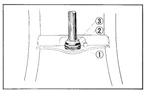
① Dust seai washer ② Dust seal ③ Steering bottom cone race
