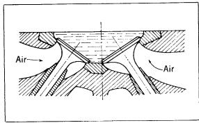
Checking the valve seat contact Fig. 48
