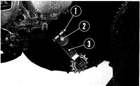
① 6 mm bolt ② Tensioner shaft ③ Tensioner Fig. 38
