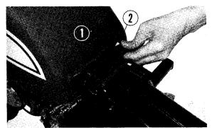
① Fuel tank ② Fuel tank band Fig. 11
