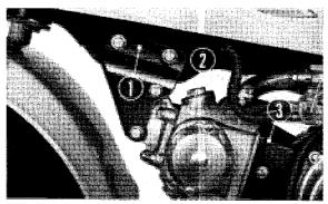
① Engine mounting bracket ② Cylinder head ③ Cylinder Fig. 98
