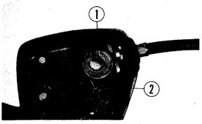
① Throttle cable end ② Throttle lever Fig. 112
