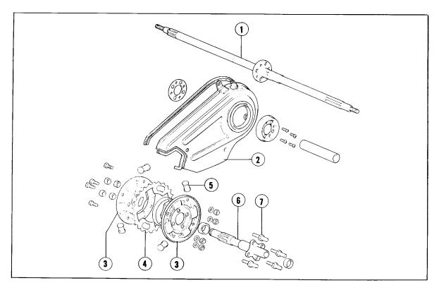
① Rear wheel axle ② Drive chain case ③ Damper holder ④ Final driven sprocket ⑤ Damper rubber ⑥ Wheel shaft ⑦ Rear drive bolt Fig. 103
