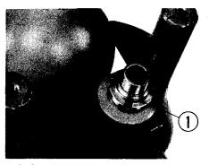
1 Steering head top thread 2 Steering stem Fig. 109
