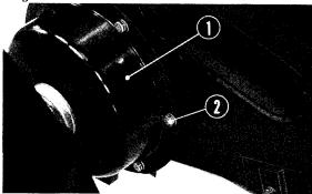
①Brake drum cover B ② 6 mm bolt
