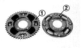
16. Remove the four 6 mm nuts and 8 mm nuts and remove the final driven sprocket assembly.
