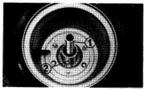
(1) Front wheel side collar (2) Front wheel hub Fig. 130
