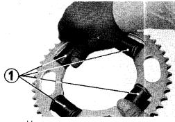
17. Remove the damper rubbers from the final driven sprocket.
