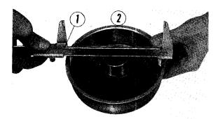
1 Vernier caliper 2 Rear brake drum Fig. 80
