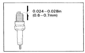
Measuring the spark gap Fig. 121
