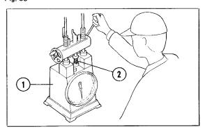
Checking the clutch spring
