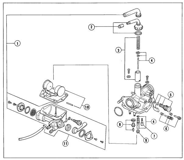
(1) Carburetor assembly (2) Top set (3) Throttle valve set (4) Jet needle set (5) Cock button set (6) Screw set (7) Slow jet (8) Float valve set (9) Main jet (10) Float set (11) Float chamber set Fig. 100
