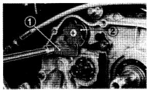
(1) Shift drum stop plate (2) Shift drum stop
