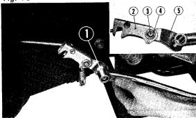
① Brake pedal② Escape lever③ Escape shaft④ 2 mm split pin⑤ Brake pedal
