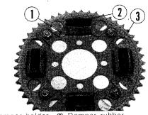
① Damper holder ② Damper rubber ③ Final driven sprocket assembly
