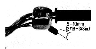
To adjust the throttle cable free play, remove the rubber sleeve and turn the cable adjuster in or out until the correct free play is obtained.
