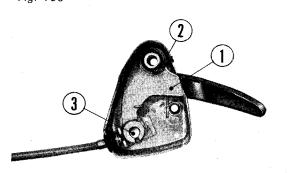
① Throttle lever ② Snap ring ③ Throttle cable end
