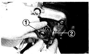
6. Pull up the sub transmission shift fork and remove the sub transmission low gear.
