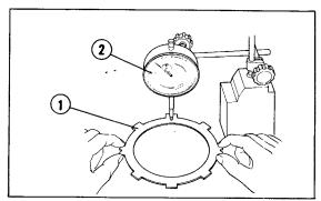
Checking the clutch plate (1) Clutch palte (2) [Fig. 88 (2) Dial gauge
