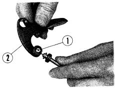
① Throttle cable ② Throttle lever Fig. 65
