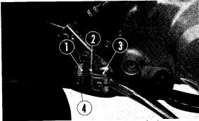
(1) Brake pedal spring (2) Tensioner lock arm
