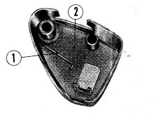
① Throttle lever spring ② Throttle lever case
