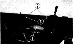
① Ignition coil ② 5 mm nuts ③ 5 mm spring washers
