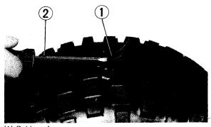
(1) Rubber plug(2) Inserting needle
