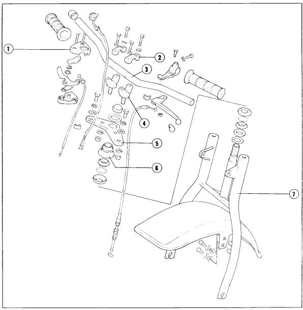
① Throttle lever cover ② Upper holder ③ Steering handle pipe ④ Lower holder ⑤ Fork top bridge plate ⑥ Steering head top thread ⑦ Front fork Fig. 104
