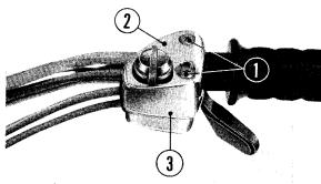
① Screw ② Throttle lever cover ③ Throttle lever case Fig. 106
