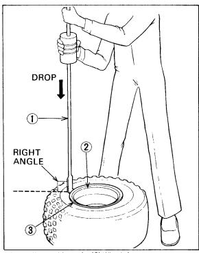
(1) Tire disassembly tool (2) Wheel rim
