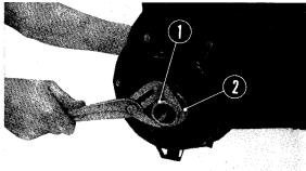
① Brake drum nut ② Seal washer Fig. 52
