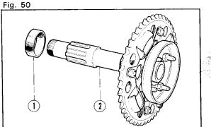
① Wheel shaft collar ② Wheel shaft
