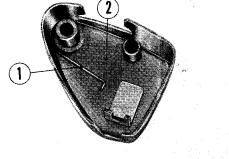
2. Apply grease to the end of the throttle cable, and then connect it to the throttle lever.
