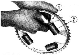
① Final driven sprocket ② Damper rubber Fig. 45
