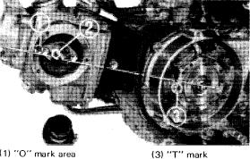
12. Make sure that the camshaft pin hole in the cam sprocket is facing toward the groove in the cylinder head when the "T" mark on the rotor is aligned with the mark on the stator. Also make sure that "O" mark on the cam sprocket is facing in the same direction for the reinstallation.
