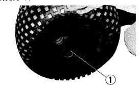
4. Repair punctures with a rubber plug.
