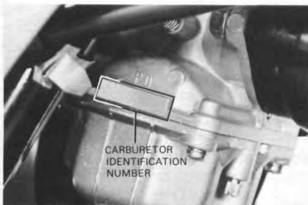
The carburetor identification number is on the carburetor body right side.
