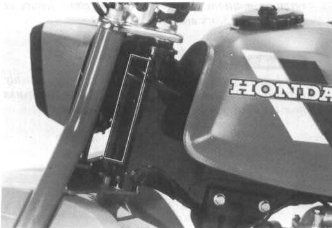
The frame serial number is stamped on the steering head left side.
