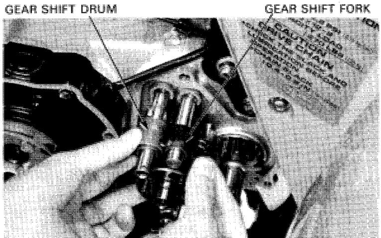
Install the low gear onto the drive shaft and install the plain washer.
