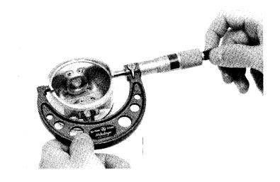
Measure the piston pin hole I.D.
