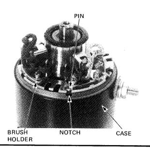
Install the rear cover aligning its slot with the brush holder pin.
