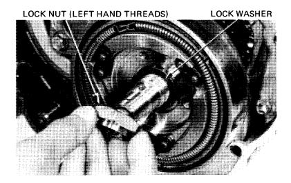
Hold the recoil starter driven pulley with a screw-driver or suitable lever (Page 9-7).
