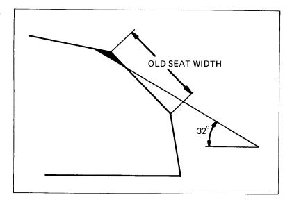
Use a 60 degree cutter to remove the lower 1/4 of the old seat. Remove the cutter and inspect the area you have just cut.
