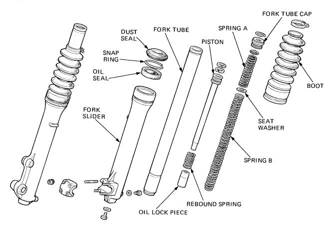
Install the rebound spring and piston into the fork tube.
