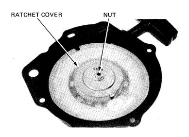
Remove the ratchet, ratchet guide, spring seat and spring.
