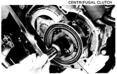
LOCK NUT WRENCH, 30 mm Equivalent commercially 07907–6890100 available in U.S.A.
