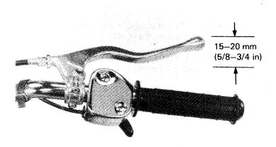
Adjust free play by turning the adjusting nut.
