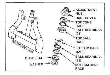
Drive new top and bottom ball races into head pipe with the special tools.
