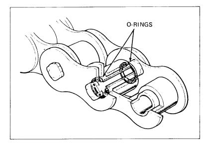
Clean the drive chain with kerosene and wipe dry.
