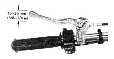
Adjust the lever and pedal free play by turning the adjusters at the lower end of the cables.
