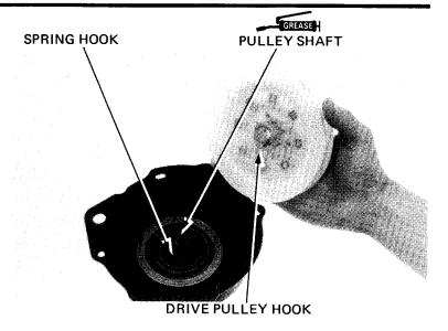
Preload the starter spring by turning the pulley 2 turns clockwise.
