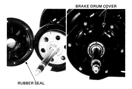
Tighten the brake drum inner nut.
