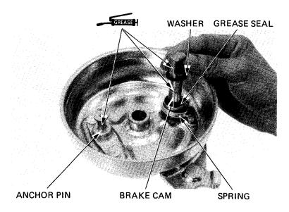
Insert the end of the spring into the hole in the brake cam.
