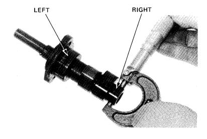
Using a micrometer, measure the height of each cam lobe and inspect it for wear or damage.
