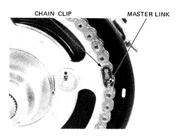
The drive chain is equipped with grease-retaining O-rings inside the chain to improve its service life. However, special precautions must be taken when adjusting, lubricating, washing and replacing the chain.
