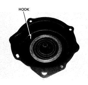
Apply grease to the pulley shaft and install the drive pulley by hooking the end of the spring on the drive pulley hook.
