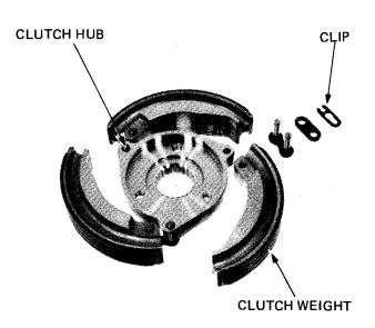
Install the centrifugal clutch springs, using a screw-driver.
