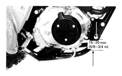
Measure the rear brake lever (parking brake) free play at the end of the brake lever.
