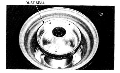
Install the brake drum onto the wheel hub using new lock washers and the bolts.
