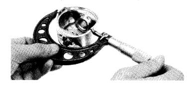
Measure the piston pin hole I.D.
