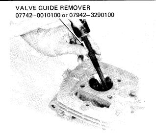
Install an O-ring on the new valve guide. Drive in the guide from the top of the head.
