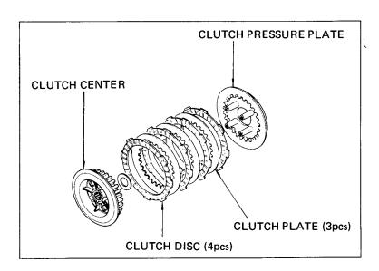
Install the thrust washer and clutch assembly.
