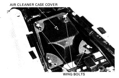
Remove the air cleaner element assembly from the air cleaner case.
