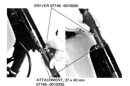
Apply grease to the top and bottom ball races and install 21 ball bearings for both the top and bottom ball races.
