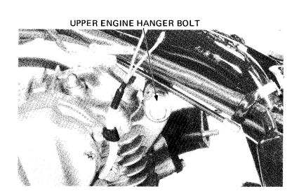
Remove the front engine hanger bolts and plates.
