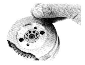
Measure the pump tip clearance.
