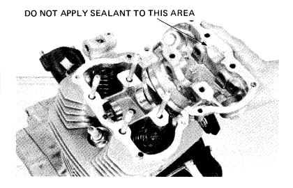
Coat the camshaft bearing and bushing with molybdenum disulfide grease.
