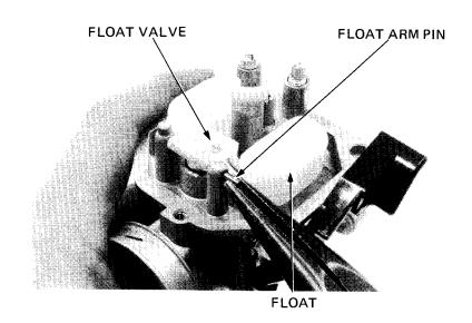
Inspect the float valve and seat for wear or damage. Replace them as a set if wear or damage can be seen.
