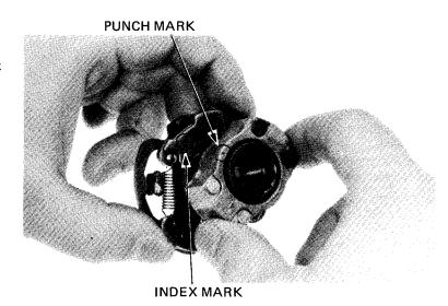
Install the dowel pin and pulse rotor/advancer assembly.
