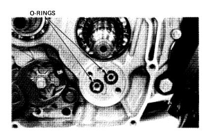
Align the oil pump driven gear holes with the gear cover holes and install the oil pump assembly.
