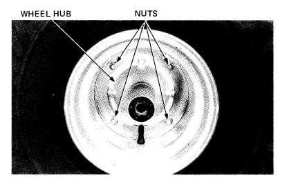
Make sure the dust seal on the wheel hub is in good condition.
