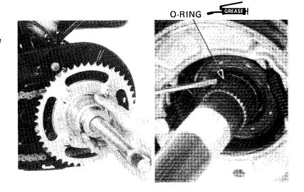
Install the brake drum.
