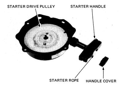
Remove the starter rope from the drive pulley. Check the starter rope for wear or damage.
