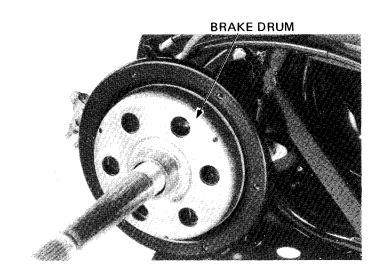
Make sure that the dust seal on the brake drum cover is in good condition.
