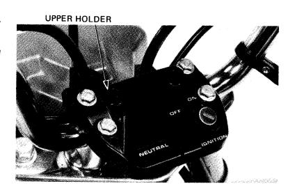
Install the front and rear brake lever brackets and holders on the handlebar and tighten the screws lightly.
