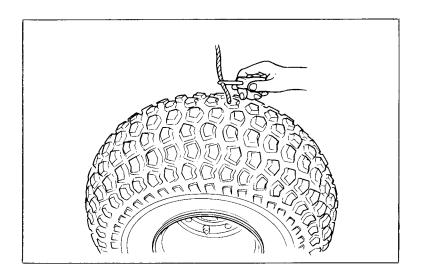
If a plug has been inserted, trim it even with the inner tire surface.
