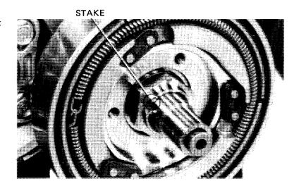
Place the oil filter rotor cover gasket onto the clutch hub.
