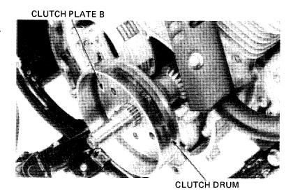
Remove the one-way clutch center and sprag.
