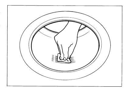
Apply cement over the area marked and allow it to dry. Remove the lining from the patch and center it over the injury.
