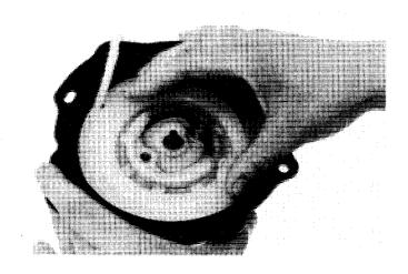
Route the rope end through the starter housing hole and install the handle.
