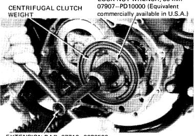
EXTENSION BAR 07716-0020500 (Equivalent commercially available in U.S.A.)
