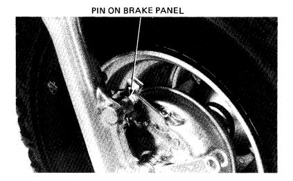
Clean the axle shaft and holder. Install the holder with "UP" facing upwards. Install the axle holder nuts but do not tighten at this time.
