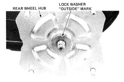
Tighten the rear axle nuts.
