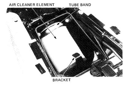
Wash the element in non-flammable or high flash point solvent, squeeze out the solvent thoroughly, and allow to dry.
