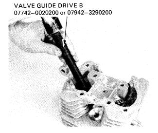
Ream the new valve guide after installation.
