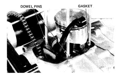
Coat the cylinder bore and piston rings with engine oil and install the cylinder.
