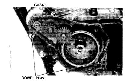
Install the left crankcase cover using the six bolts.
