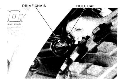
When the drive chain becomes extremely dirty, it should be removed and cleaned prior to lubrication.
