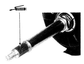
Install the rear wheel hubs over the axle.
