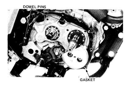
Install the right crankcase spacer and tighten it with the four bolts.
