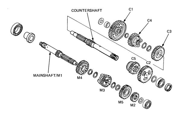
Install the mainshaft and countershaft assemblies into the right crankcase.
