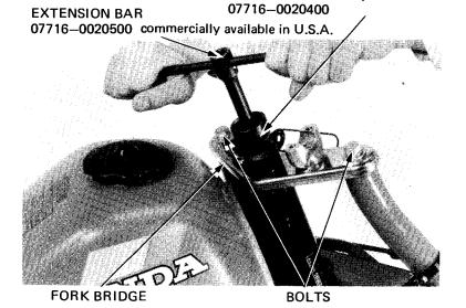
Remove the steering adjustment nut.
