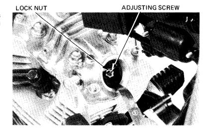
Adjust by loosening the lock nut and turning the adjusting screw until there is a slight drag on the feeler gauge.
