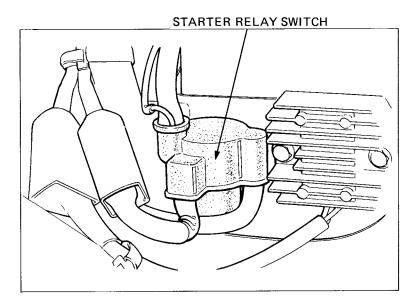
Connect an ohmmeter to the starter relay switch terminals.
