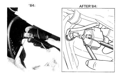
Measure the secondary coil resistance with the spark plug cap in place.
