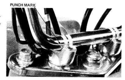
Install the handlebar upper holders on the handlebar.
