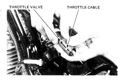
Remove the needle clip retainer, jet needle and needle clip. Inspect the throttle valve and jet needle surfaces for dirt, scratches or wear.
