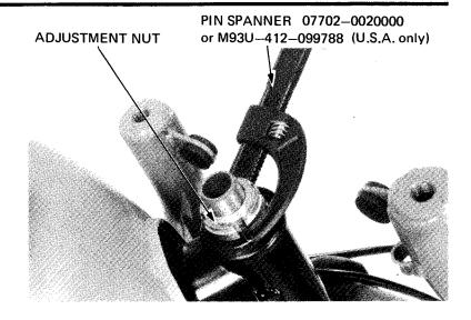
Remove the top cone race, ball bearings and front fork being careful not to drop the bearings.
