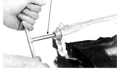
Remove the dust seal and the snap ring. Remove the oil seal.
