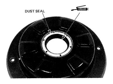
Install the rubber seal onto the brake drum cover.
