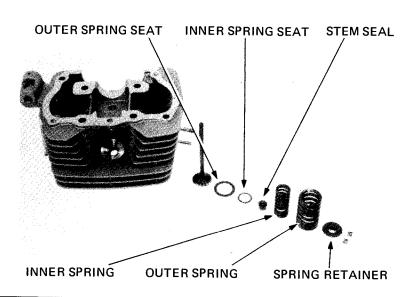
Install the valve spring retainers and install the valve cotters.
