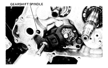
Remove the thrust washer, circlip and disassemble the gearshift spindle.
