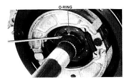
Drive the rear axle out from the right side using a soft hammer.
