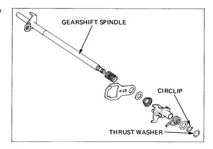
Remove the drum stopper plate and drum stopper arm.
