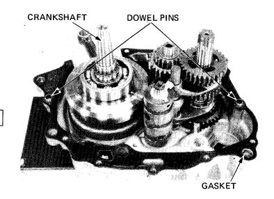
Tighten the left crankcase 6 mm bolts in a criss-cross pattern.
