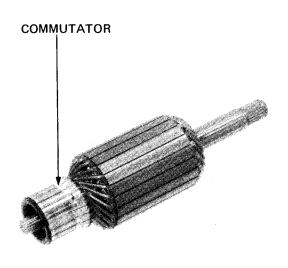
Check for continuity between pairs of commutator bars. Also, make a resistance check between individual commutator bars and the armature shaft. There should be no continuity.
