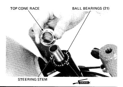
Install the bearing adjustment nut and dust cover and tighten it snug against the top cone race. Then, back it off 1/8 turn.
