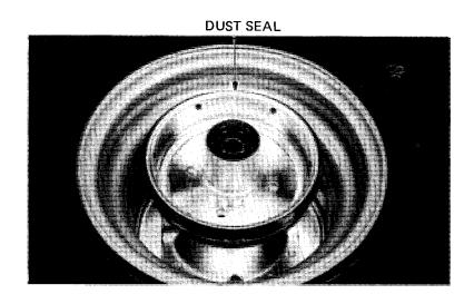
Remove the front wheel hub nuts and hub.
