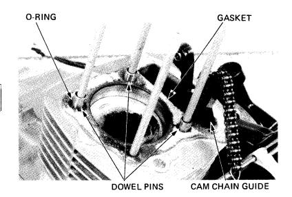
Clean off any gasket material from the cylinder surface.
