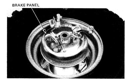
Bend down the lock washer tabs and remove the brake drum bolts and drum.
