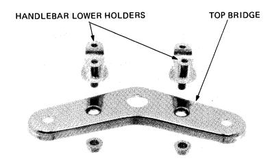
Install the steering stem nut and fork bridge bolts. Tighten the stem nut.
