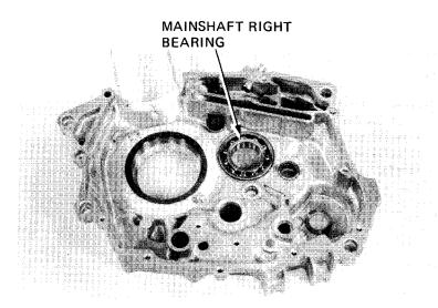
Drive the bearings into the right and left crankcases with the following tools:
