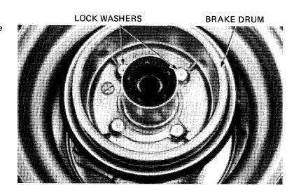
Remove the brake panel dust seal.
