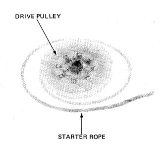
Check the recoil starter spring. Remove the spring if it is broken.
