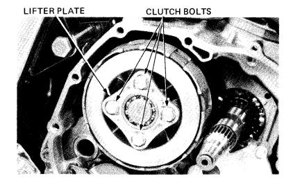
Install a CLUTCH CENTER HOLDER as shown, and remove the clutch lock nut.
