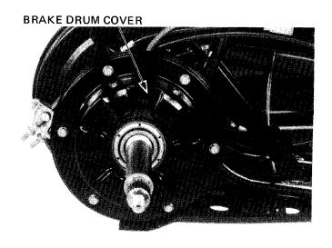
Remove the brake drum.
