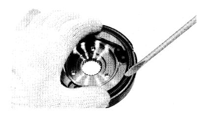
Install the centrifugal clutch weight assembly onto the clutch drum.
