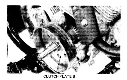
Attach the centrifugal clutch weights to the clutch hub with the links and clips.
