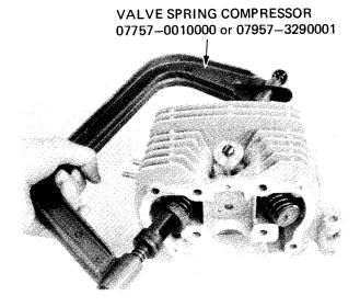
Tap the valve stems gently with a plastic hammer to firmly seat the cotters.
