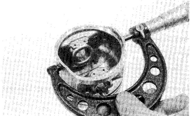
Measure the piston pin hole I.D.
