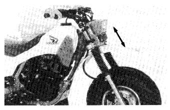
Raise the front of the vehicle so that there is no weight on the front wheel.
