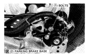
Remove the boot and parking brake shaft from the brake base.
