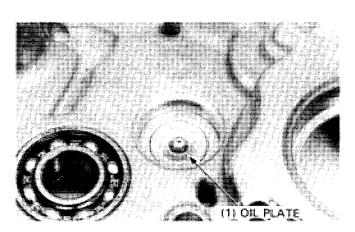
Place a new mainshaft bearing with the sealed end facing down.
