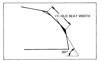
Install a 45 degree finish cutter and cut the seat to the proper width. Make sure that all pitting and irregularities are removed. Refinish if necessary.
