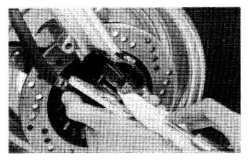
Install the caliper to the front fork so the disc is positioned between the pads, being careful not to damage the pads. Tighten the caliper mounting bolts.
