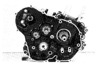
Place the engine with the left crankcase down and remove the right crankcase while tapping the cases at several locations with a soft hammer.
