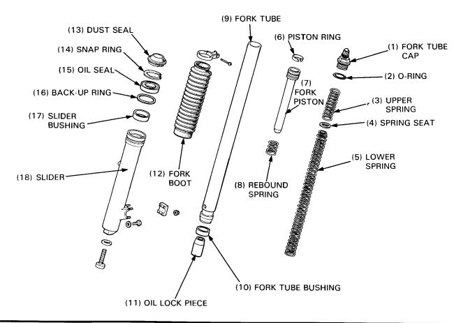
Install the piston ring on the piston.
