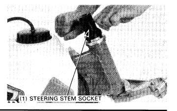
Remove the steering bearing adjustment nut, steering stem, upper cone race and steel balls.
