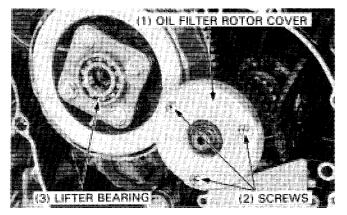
Unstake the oil filter rotor lock nut with a drill or grinder. Be careful not to damage the crankshaft threads.
