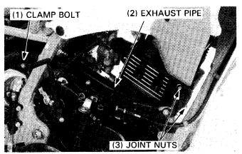
Remove the exhaust muffler mounting bolts and the exhaust muffler.
