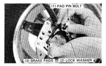
Tighten the pad pin bolts.
