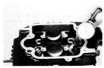
If the stem-to-guide clearance exceeds the service limits, determine if a new guide with standard dimensions would bring the clearance within tolerance. If so, replace any guides as necessary and ream to fit.
