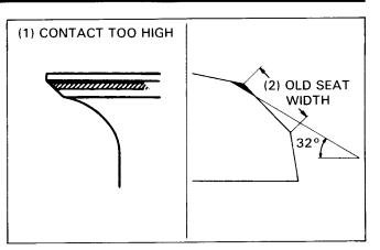
If the contact area is too low on the valve, the seat must be raised using a 60 degree inner cutter.
