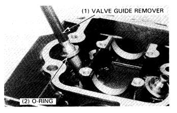
Inspect the valve guide for damage.
