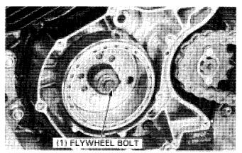
Remove the flywheel with the puller, then remove the woodruff key from the crankshaft.
