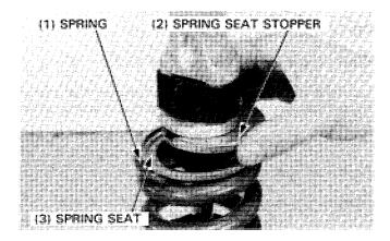
Turn the adjusting nut to obtain the correct spring length.
