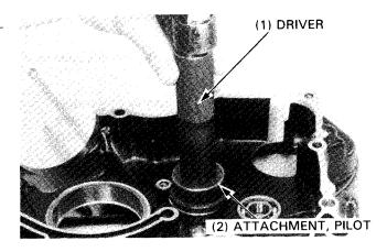
Drive new bearings into the right crankcase using the following tools:
