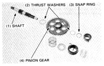
Install the ratchet over the shaft aligning its wide groove with the punch mark on the shaft.
