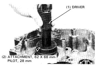
Install the crankshaft into the left crankcase using the special tools.
