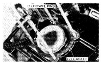
Stagger the piston ring end gaps 120° a part. Coat the cylinder bore and piston rings with engine oil and install the cylinder.
