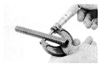
Check that the fork shaft is not bent, worn or damaged.
