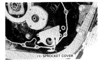
Remove the snap ring and the oil pump driven sprocket from the shaft.
