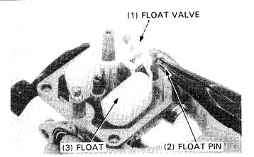
Inspect the float value and value seat for grooves, nicks or contamination.
