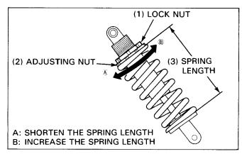
Tighten the lock nut while holding the adjusting nut.
