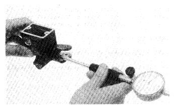
Check the piston for scratches, scoring or other damage. Check the primary and secondary cups for wear, deterioration or damage.
