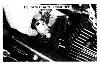
Install the sealing washer and bolt, and tighten the bolt securely.
