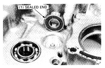
Drive in a new mainshaft bearing with the sealed end facing down.
