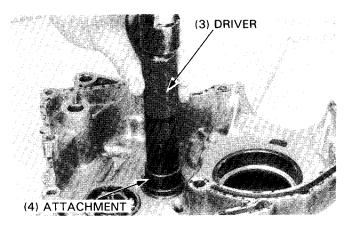
Drive in a new countershaft bearing.
