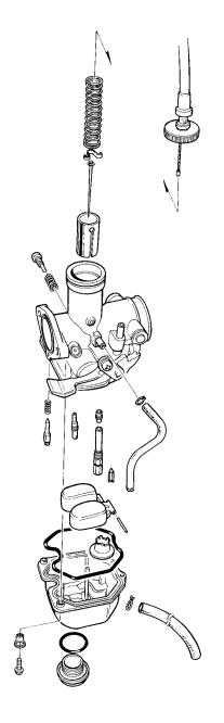
Remove the float chamber from the carburetor body.
