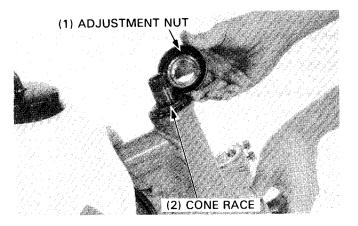
Check the cone and ball races for wear or damage and replace if necessary.
