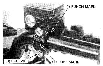
Position the throttle housing on the handlebar and install it using the throttle housing holder and two screws.
