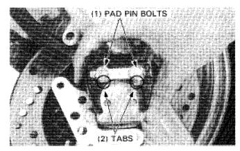
Remove the pad pin bolts, lock washer and brake pads.
