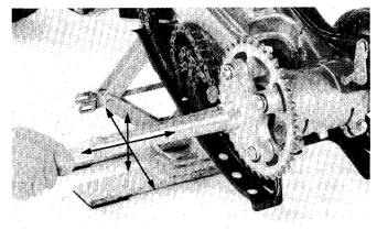
Remove the nuts, chain guide plate, bolts and sprocket from the sprocket hub.
