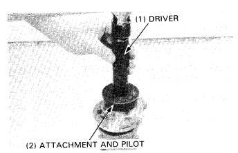
Apply grease to the lip of new dust seals and drive the dust seals into the bearing holder until their outside surfaces are flush with the end surfaces of the holder.
