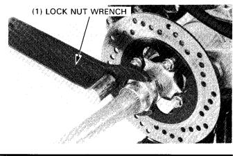
Apply a thread locking agent to the inner lock nut threads.
