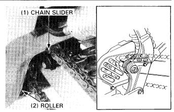
When the depth of the grooves in the slider reaches 2.0 mm (0.08 in), remove material to lower the height of the center ridge between the grooves to less than 2.0 mm (0.08 in).
