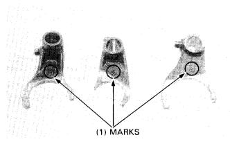
Install the shift drum and align each shift fork guide pin with its guide groove in the drum.
