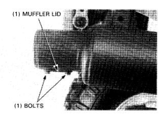
Start the engine and rev it up to blow accumulated carbon deposits out the muffler.
