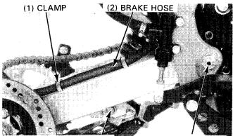
(4) LOWER MOUNT BOLT (3) PIVOT BOLT, NUT
