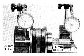
Measure the axial clearance of the connecting rod big end.
