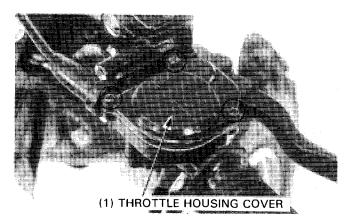
Loosen the throttle cable adjuster and remove the lock nut.
