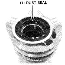
Remove the bearings, spacers and center spacer from the bearing holder.
