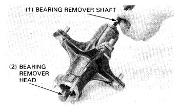
Remove the wheel bearings with a bearing remover.
