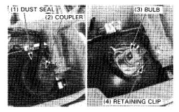
Replace the faulty bulb with a new one.
