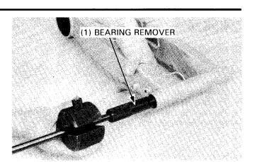
Press new needle bearings in with the side collars as shown.
