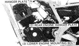
Place a floor jack or other adjustable support under the engine. Remove the top, front and rear engine hanger plates and the
