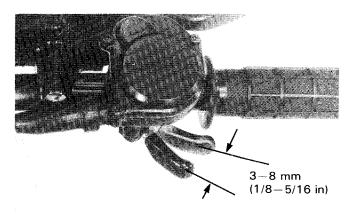
To adjust the free play slide back the rubber cap, loosen the lock nut and turn the adjuster.
