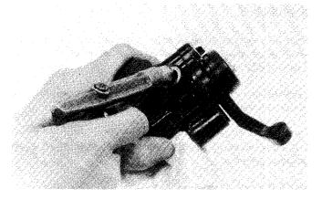
Push the dust and piston seals in and lift them out. Clean the seal grooves with clean brake fluid.
