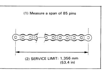
Clean the chain with kerosene. Wipe dry and lubricate only with SAE #80 or #90 gear oil. Commercial chain lubricants may contain solvents which could damage the rubber O-rings.
