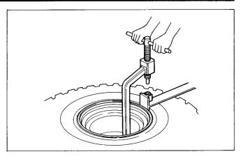
Screw in the breaker arm compressor bolt to break the bead from the tire.
