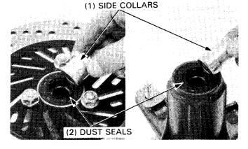
Remove the front brake disc from the wheel hub.
