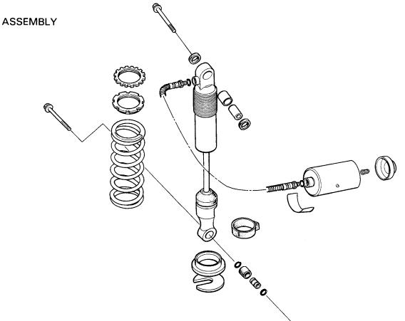
Hold the upper shock mount in a vise with soft jaws or a shop towel. Point the hole straight up.
