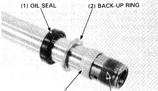
(4) SLIDER BUSHING (3) FORK TUBE BUSHING
