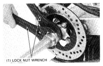
Temporarily install the left wheel hub and wheel.
