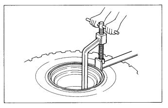
If the bead breaking is difficult with the narrow end (A side) of the breaker arm, use the wide end (B side) of the arm and repeat the procedure above.
