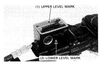
Check the front and rear brake fluid reservoir levels.
