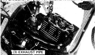
Install the top engine hanger plates and bolts. Tighten the bolts
