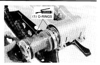
Install the bearing holder into the swingarm as shown in the figure.
