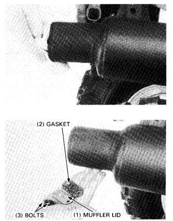
Be sure that the muffler lid bolts and gasket are in good condition. Replace the bolts and gasket if necessary.
