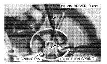
Drive out the spring pin from the lifter arm shaft and discard it. **TOOL:**
