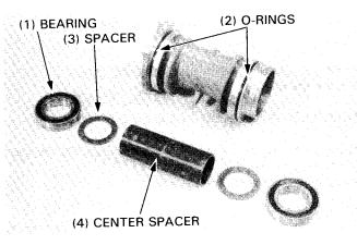
Install the spacer into the bearing holder. Drive a new right bearing into the bearing holder with common tools.
