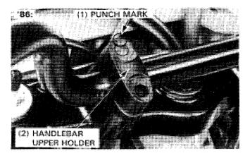
Tighten the front bolts first, then tighten the rear bolts.
