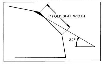
Use a 60 degree cutter to remove the bottom 1/4 of the old seat. Remove the cutter and inspect the area you have refaced.
