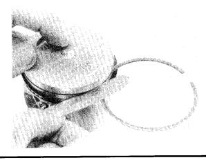
Insert each piston ring squarely into the cylinder and measure the ring end gap.
