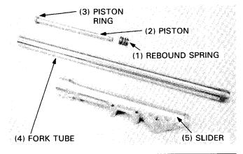
Place the fork tube in V blocks and read the runout.
