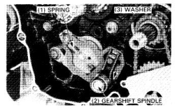
Remove the gearshift guide plate and gearshift plate.
