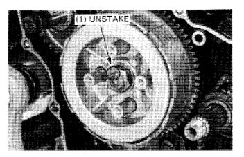
Hold the clutch center with the clutch center holder and remove the clutch lock nut.
