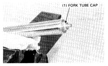
Drain the fork oil by pumping the fork up and down several times.
