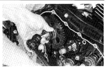
Make sure that the punch mark on the shaft faces up.
