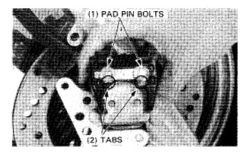
Push the caliper piston in all the way.
