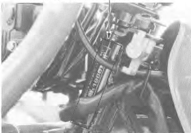
The vehicle identification number (VIN) is on the steering head's left side.
