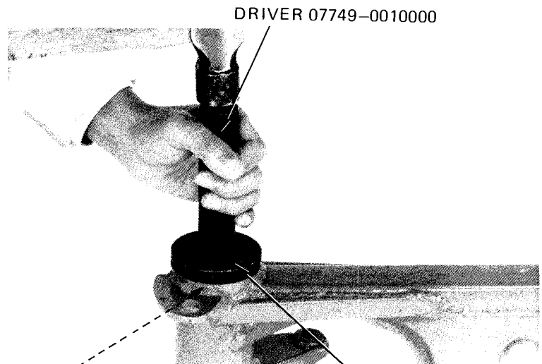
PILOT 35 mm 07746-0040800 ATTACHMENT 62 x 68 mm NEEDLE BEARING REMOVER 07746-0010500 07946-KA50000
