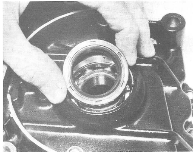
29.6b ... and renewed as a matter of course during overhaul
