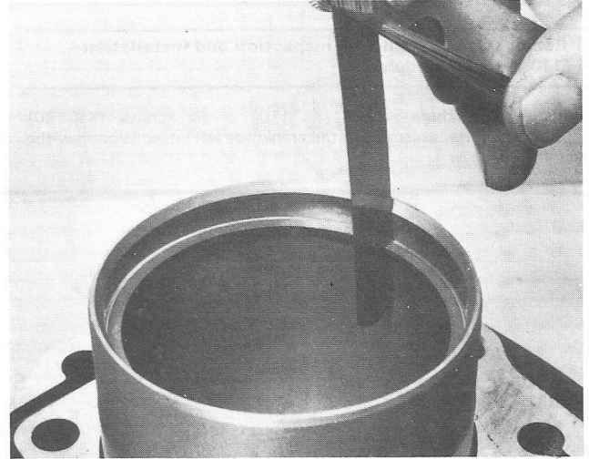
14.10 Measuring piston ring fitted end gap – use unworn part of bore
