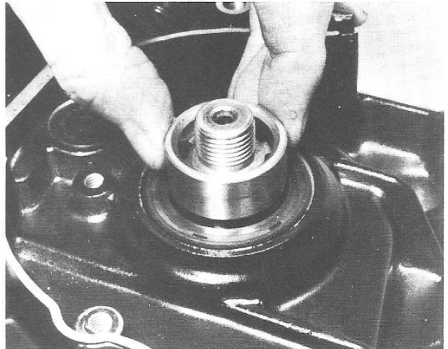
26.21 Check that all shafts rotate easily – do not forget to refit components such as output shaft collar
