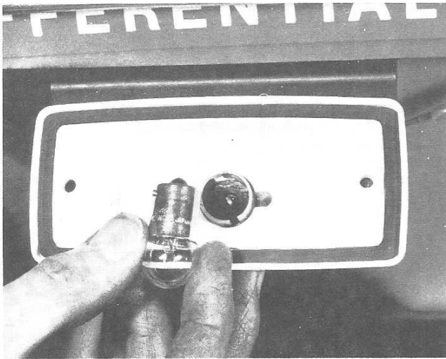
11.7b ... to remove taillight bulb
