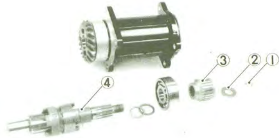
① Nut ② Washer ③ Coupling gear ④ Middle driven shaft sub-assy
